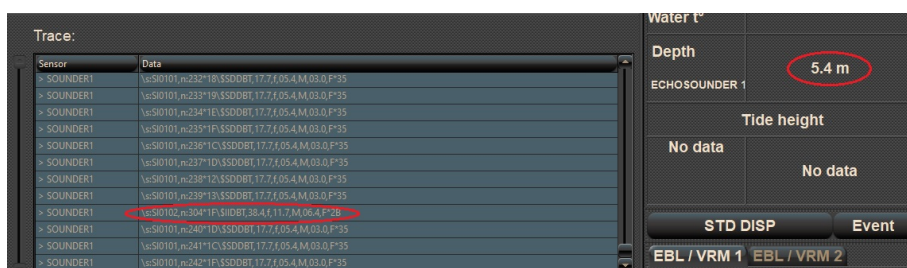
Figure 18: Original information overwritten, causing a denial of service in the navigation system
