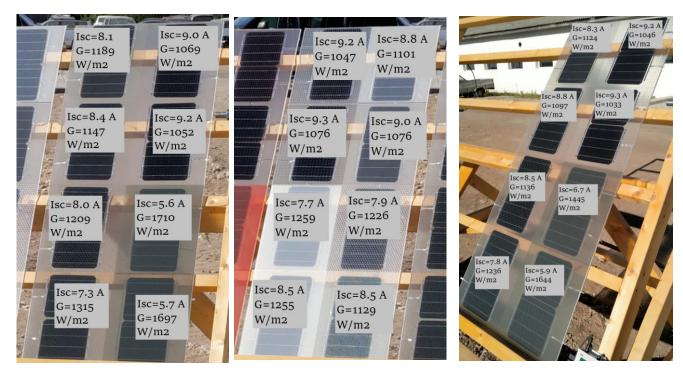
Figure 30. Power output assessments for each manufactured module.
