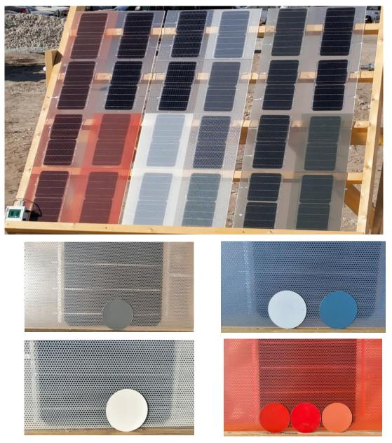
**Figure 27.** Module with digital ceramic printed front glass and coloured metal backsheet RAL code match test
