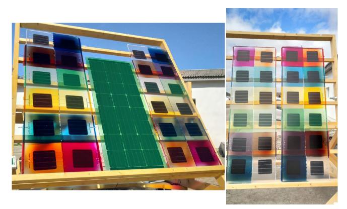
**Figure 24**. Left: Visual differences between laminating active layer of the module by using one layer EVA (on the left) and two layers of EVA foils (on the right) with green EVA encapsulated module. Right: Visual examination due to inclination changes.
