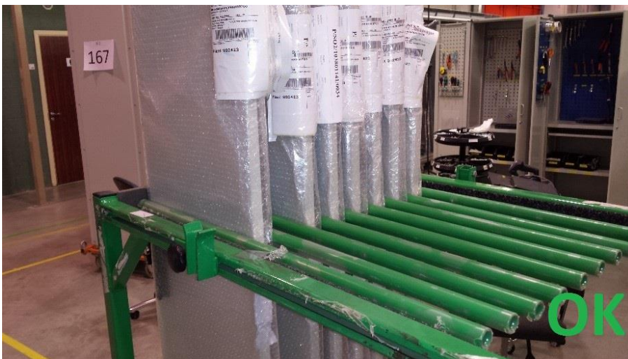
Figure 7.21. Picture of the improvement – doors are now sent in bubble-wrap (OK)
