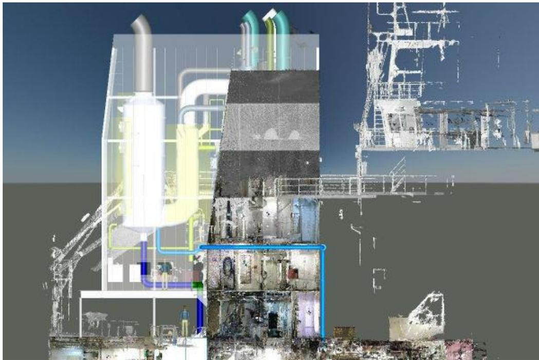
*Figure 22 Scrubber 3D model. Source: MFAME*
