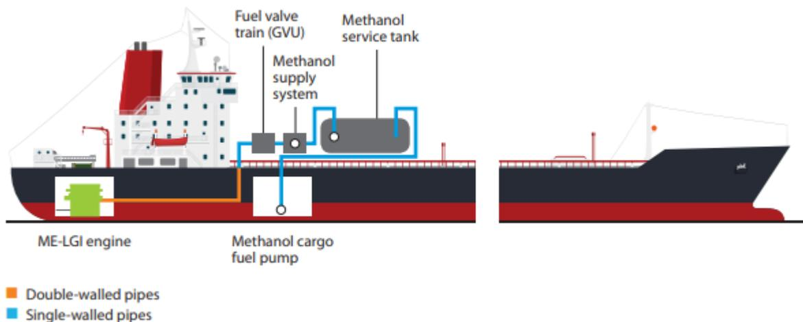
**Figure 28 Methanol Conversion. Source: MAN**
