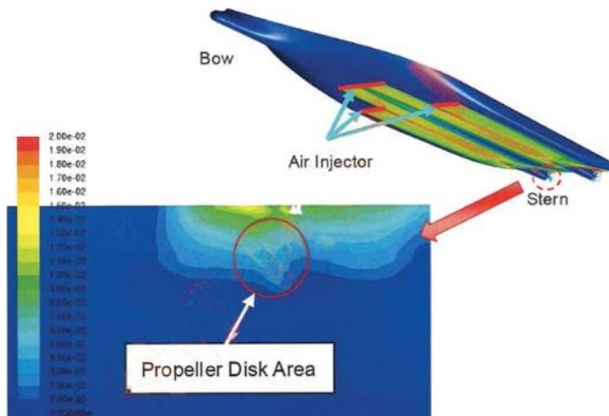
*Figure 10 Air Bubbling system. Source: Class NK*
