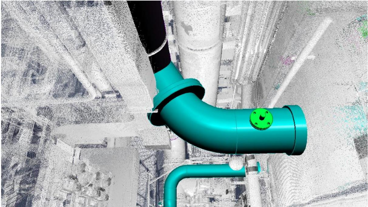
*Figure 35 Point cloud and 3D model collision. Source: Alfa laval*
