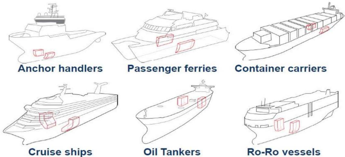
**Figure 27 LNG tank locations for various ship types. Source: Bureau Veritas**
