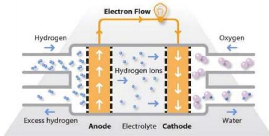
*Figure 8 PEMFC principle. Source: DNV GL*
