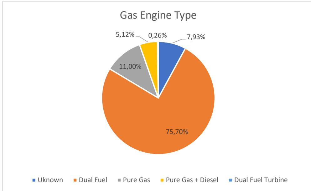
**Figure 5 LNG engine types. Source: Adapted from DNV AFI**
