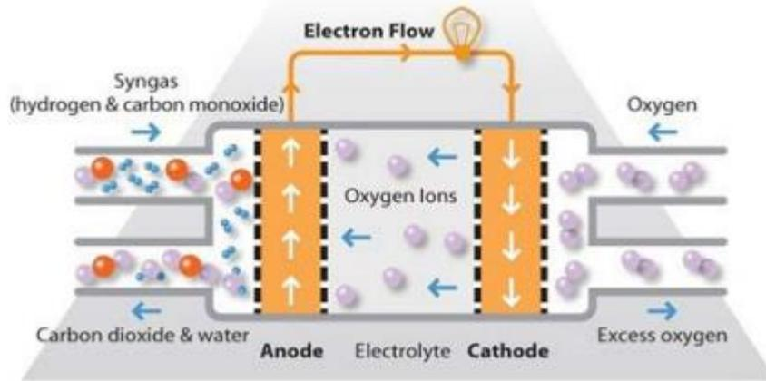
*Figure 6 SOFC principle. Source: DNV GL*
