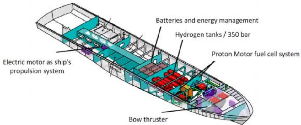
*Figure 7 FCS AlsterWasser. Source: DNV GL*
