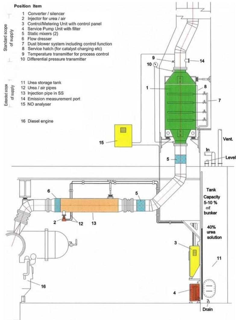
**Figure 26 Installation of an SCR. Source: Springer**
