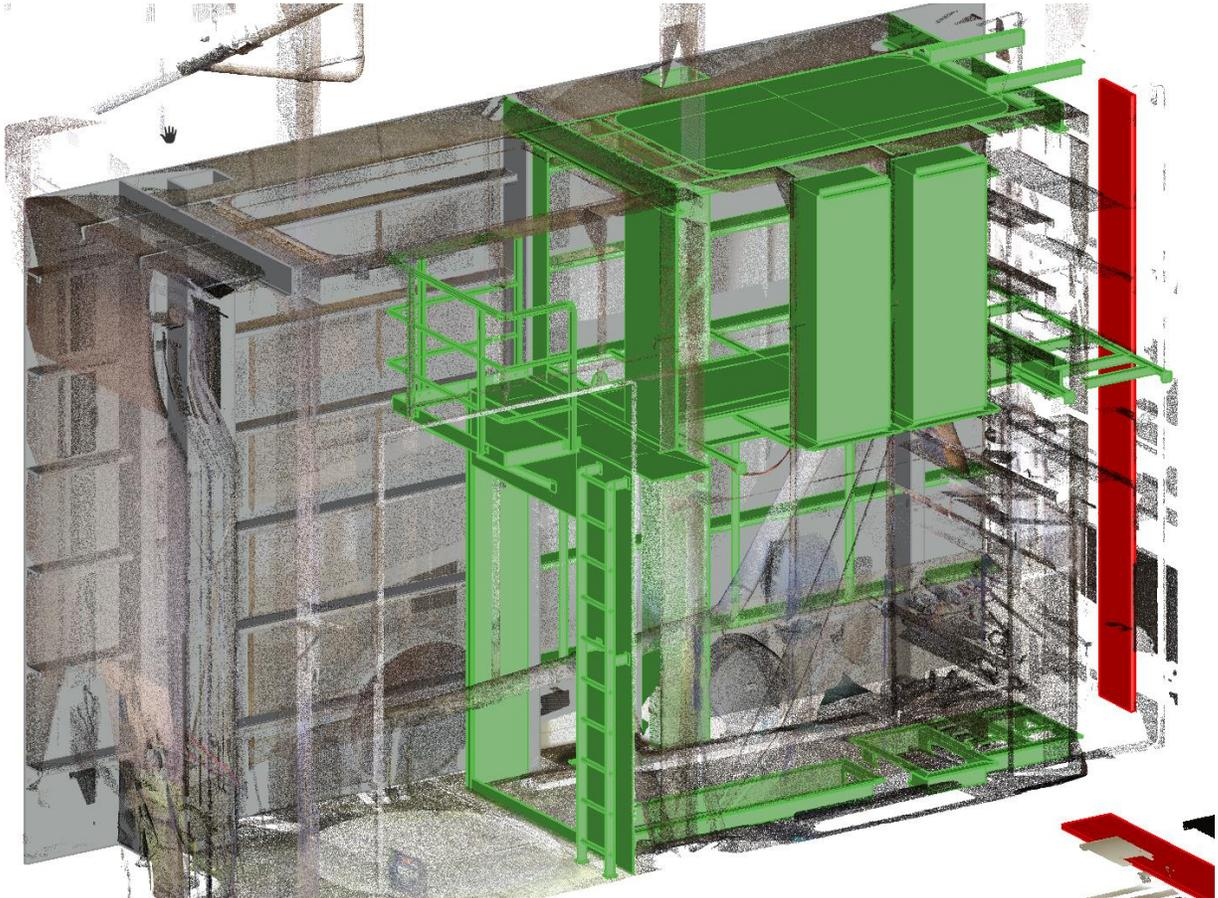
*Figure 34 New model inside a point cloud. Source: Author*
