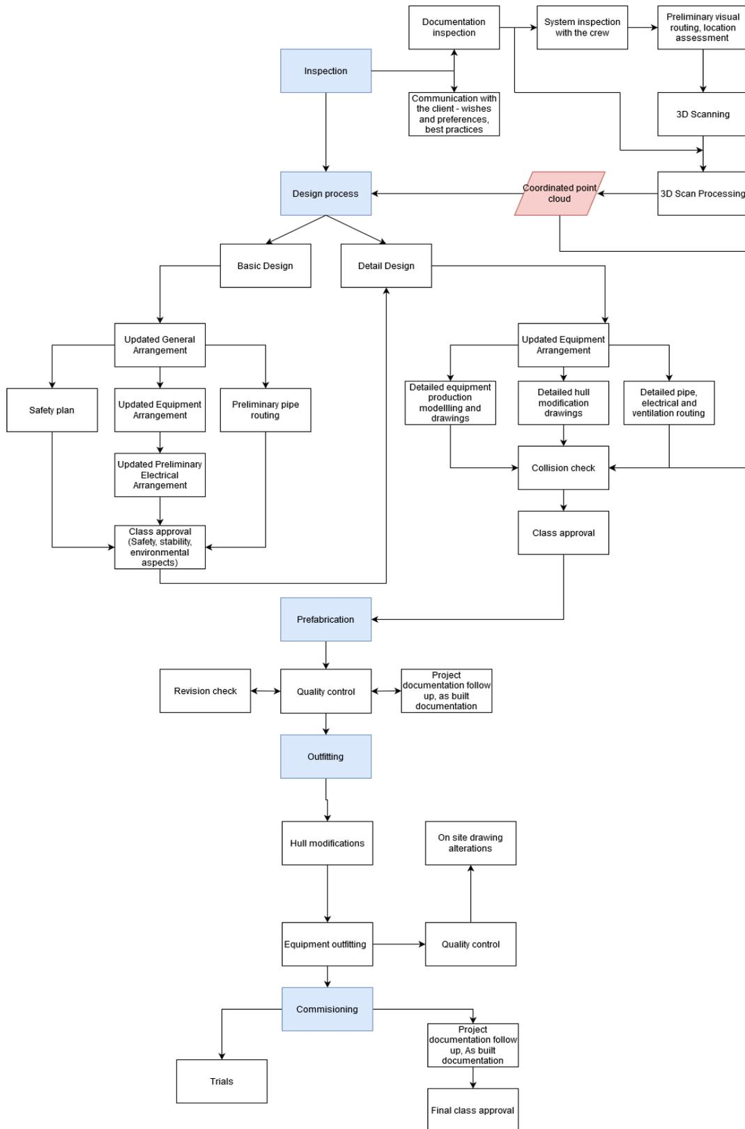
**Figure 20 Retrofit process flowchart**
