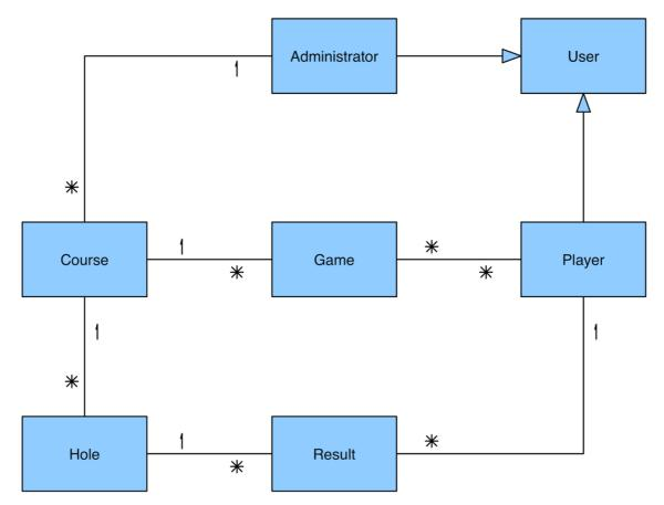
Figure 1. Conceptual entity diagram.
