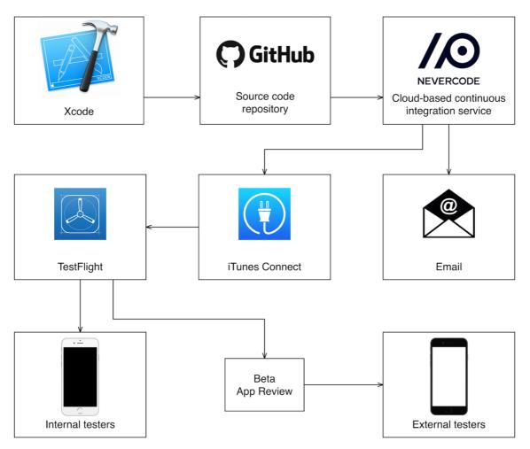
Figure 13. Continuous integration process diagram.
