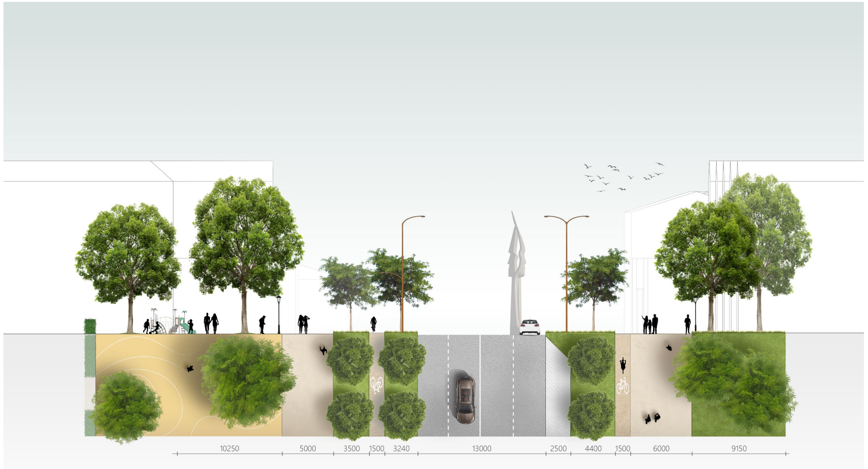
Drawing 3. Section of Narva main street S1
