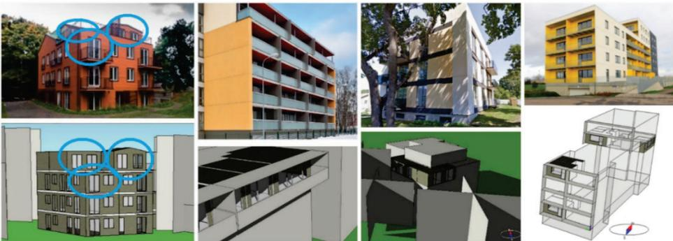
Figure 12. Example of modelled buildings with shading elements and selection of ‘critical’ rooms, which have highest potential to become overheated. Photos (top) and simulation models (bottom).
