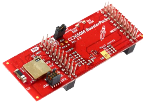
Figure 4: Texas Instruments SimpleLink™ CC2650 BoosterPack™ plug-in module [2]
