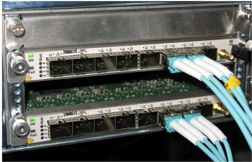
Figure 18. MTCA.4 crate with two installed FPGAs serving as a testbench.
