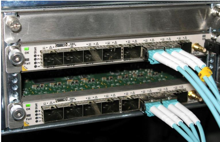
Figure 50: MTCA.4 crate with two installed FPGAs serving as a testbench.
