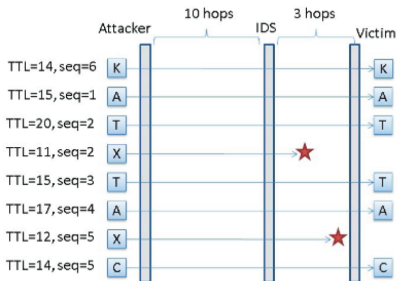
Figure 3: Duplicate insertion technique with small TTL values [39].
