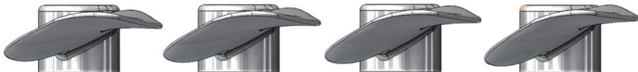
Figure 26. 254 mm (10 in) rotors with pitches 76.2 mm, 101.6 mm, 127mm and 152.4 mm (3, 4, 5 and 6 inches respectively).
