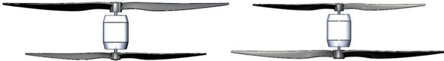
Figure 33. Pairs of coaxial rotors. Left: larger on top, smaller in the bottom. Right: smaller on top, larger in the bottom.
