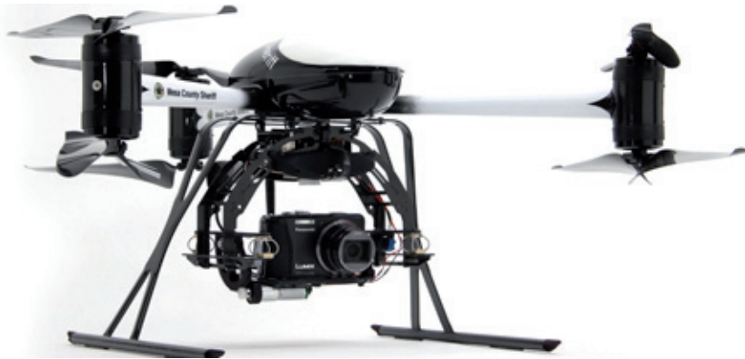
Figure 28. Draganflyer X6 with three pairs of coaxial rotors, Innovations Inc., picture from draganfly.com.
