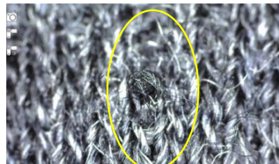
Figure 8.3.2.5 Thread break after 18 000 rubs
