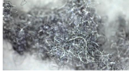
Figure 8.3.2.1 Merino wool before the abrasion test and loose wool fibres
