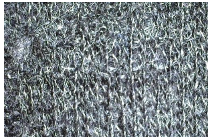
Figure 8.3.2.6 Merino wool under a microscope after 25 000 rubs
