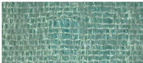
Figure 8.3.2.9 Silk after 6000 rubs, thread breakage
