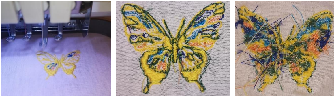
Figure 8.3.4.11 The process and results of test two embroidery on cotton fabric
