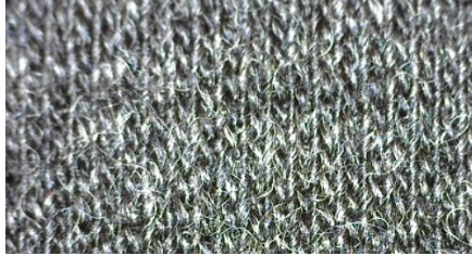
Figure 8.3.2.1 Merino wool before the abrasion test and loose wool fibres
