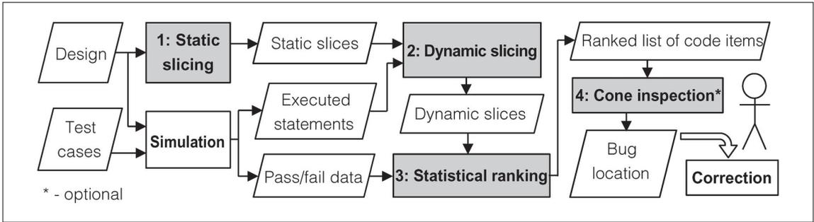
**Figure 2. Statistical bug localization flow.**
