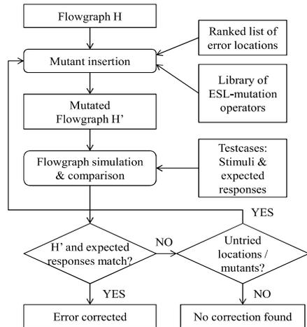
Figure 3. The mutation-based error correction flow.
