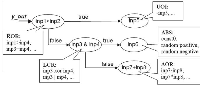
Fig. 8. “Key” mutation operators as HLDD perturbations.
