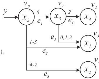
Fig. 1. Graphical representation of a HLDD for a function  $y = f(x_1, x_2, x_3, x_4)$ .
