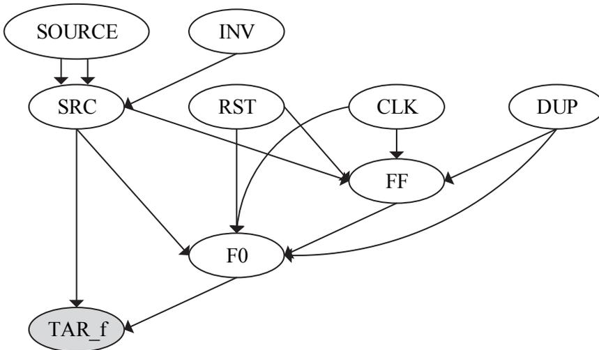
**Figure 4.9. Through-signal-assignment search based backward reference graph on the signal TAR\_f in the chopper design**
