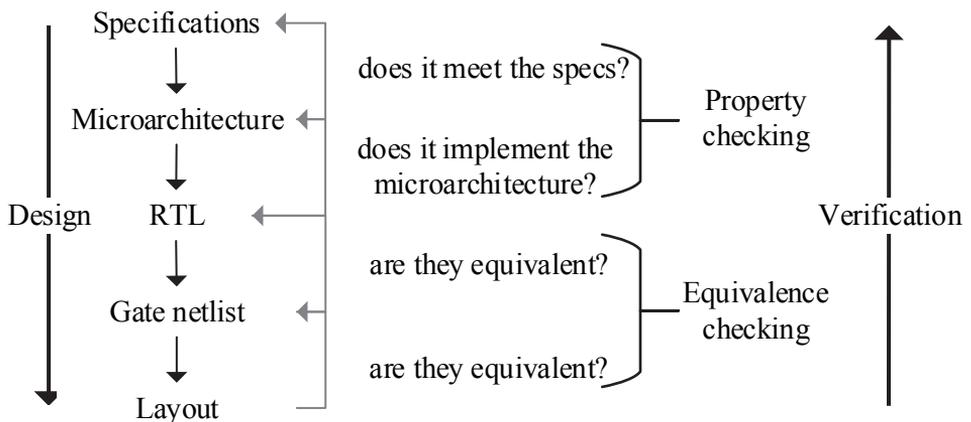
**Figure 2.2. Relationship between the design and the verification processes**
