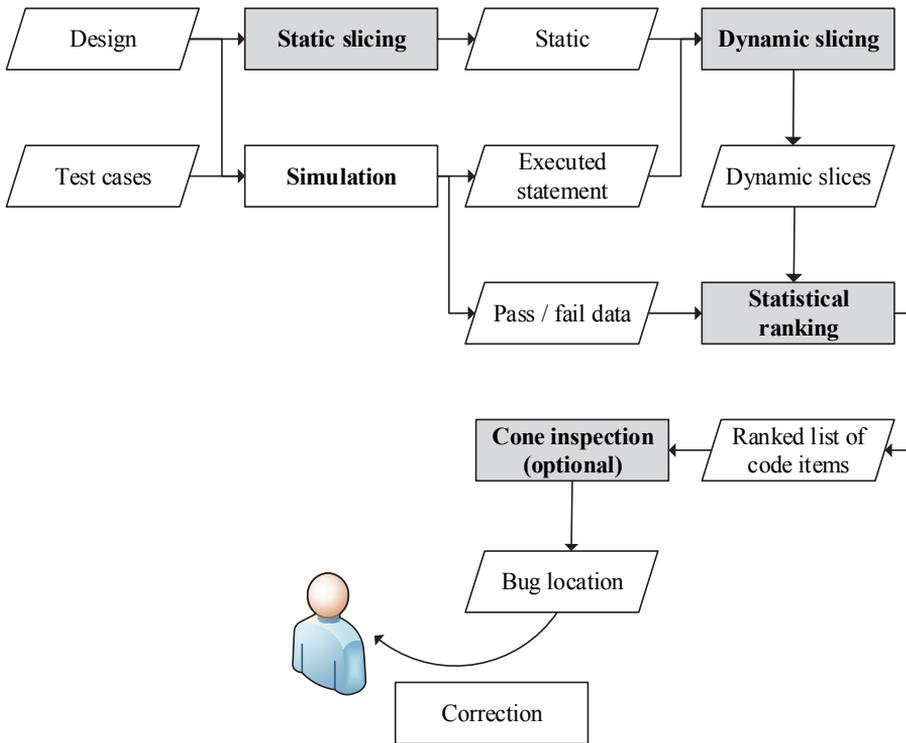
**Figure 4.6. Statistical bug localization flow**
