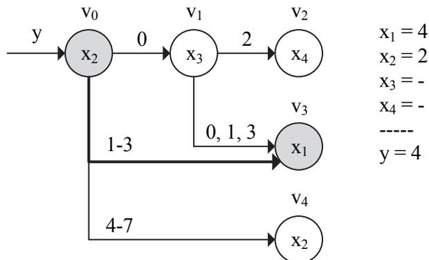
**Figure 2.7. Simulation on a decision diagram**
