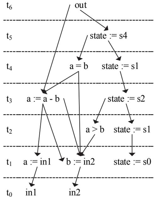
**Figure 4.3. Diagnostic tree for the passing test in Figure 4.2a**
