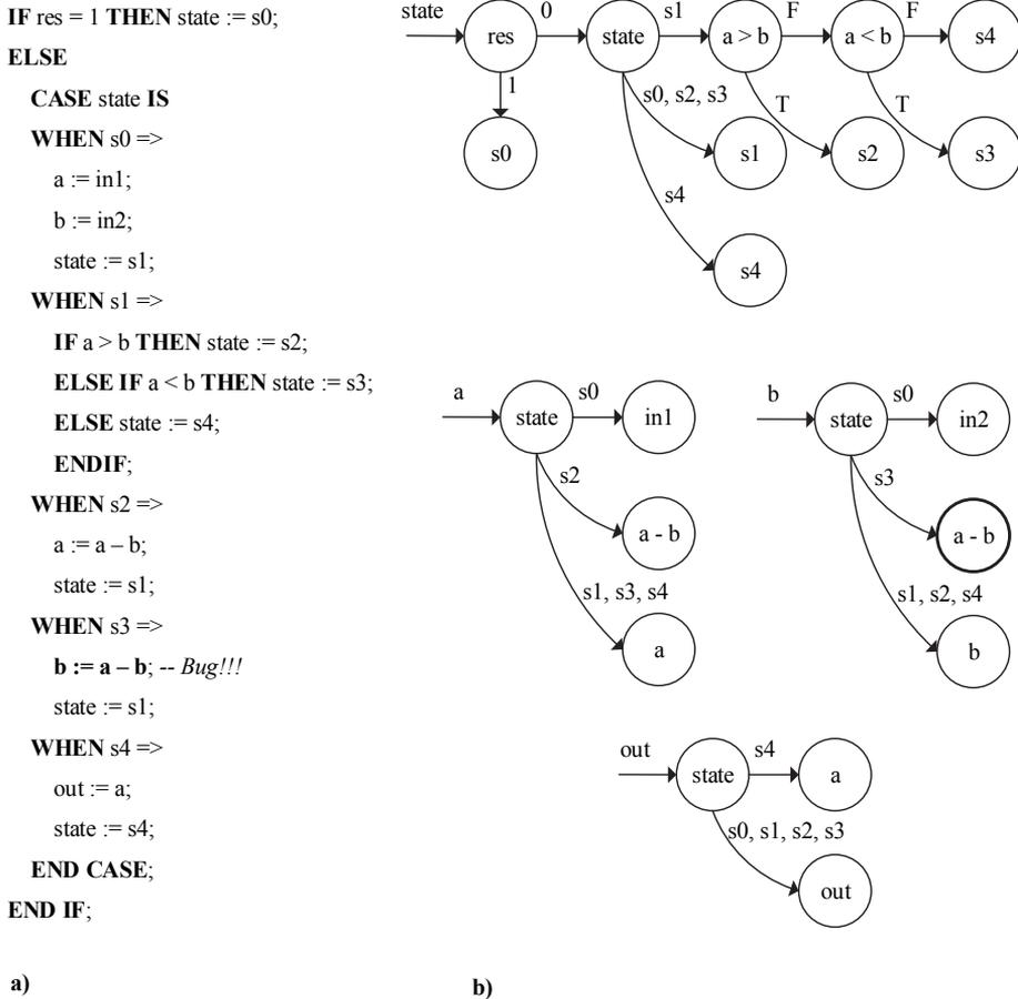
**Figure 2.10. RTL VHDL and its corresponding HLDD**
