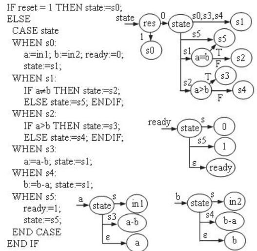
Figure 4. a) RTL VHDL and b) the corresponding HLDD
