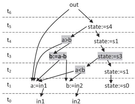
Fig. 7. Diagnostic tree for the failing test in Fig. 5b.
