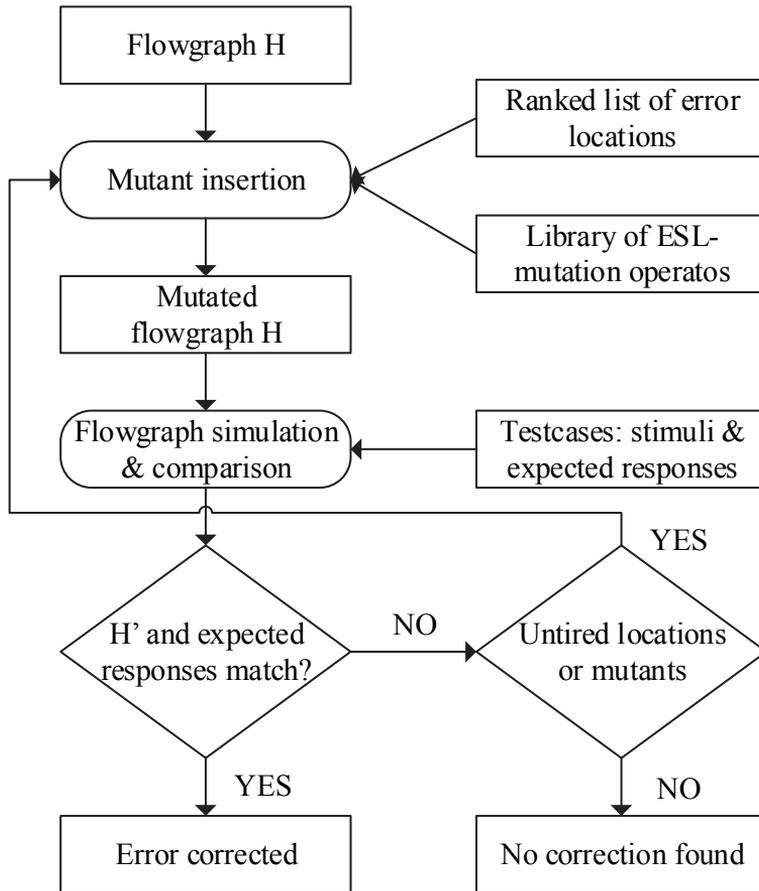
**Figure 4.13. The mutation-based error correction flow**
