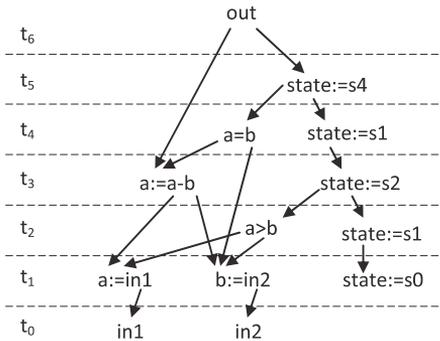
Fig. 6. Diagnostic tree for the passing test in Fig. 5a.
