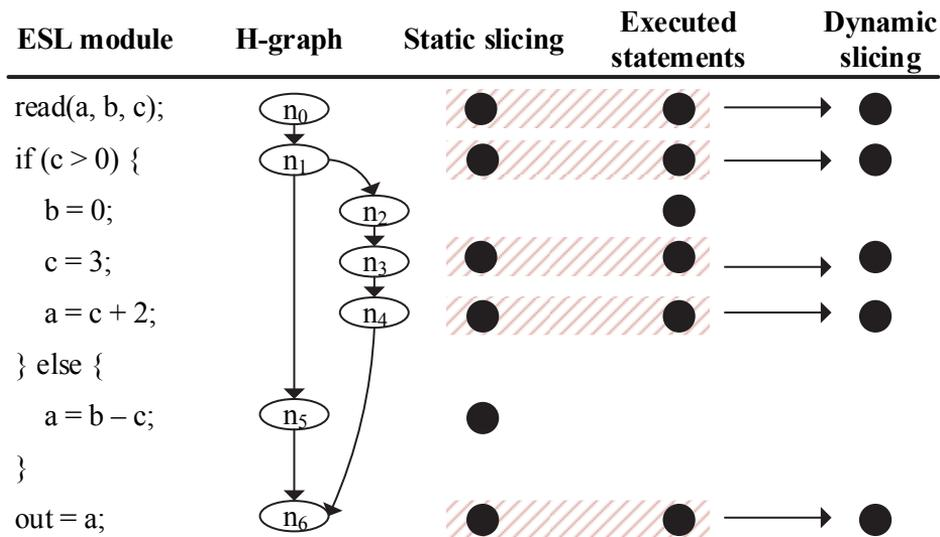
**Figure 4.12.** The ESL description is modeled as a flowgraph, i.e., hammock graph. Simulation and slicing are performed on the model representation
