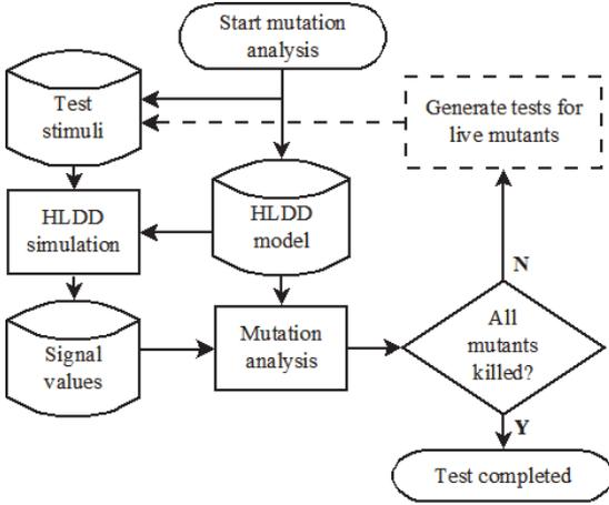
Figure 2. Data flow of the HLDD-based mutation analysis environment
