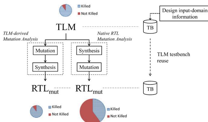
**Fig. 4** Relationship between number of mutants on the TLM and the synthesized descriptions. According to the complexity of the TLM statements, the synthesis process may produce RTL code at different levels of abstraction. Typically, a pure RTL, i.e., low level, description provides an significantly higher number of possible mutations than the corresponding high-level code
