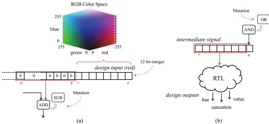
**Fig. 5** Examples of live-mutants causes for native RTL mutation analysis. **a** The mutant depends on a bit range of the integer input port which is never assigned by the testbench: by default integers
