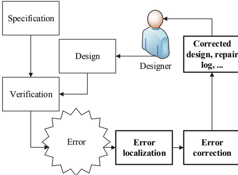
**Figure 1.4. Automated debug flow**
