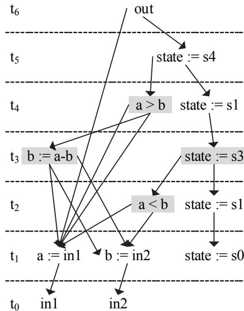
**Figure 4.4. Diagnostic tree for the failing test in Figure 4.2b**
