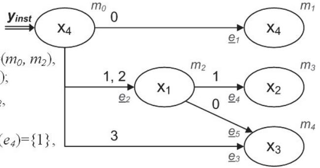
Figure 3. A high-level decision diagram representing a function  $y_{inst} = f(x_1, x_2, x_3, x_4)$
