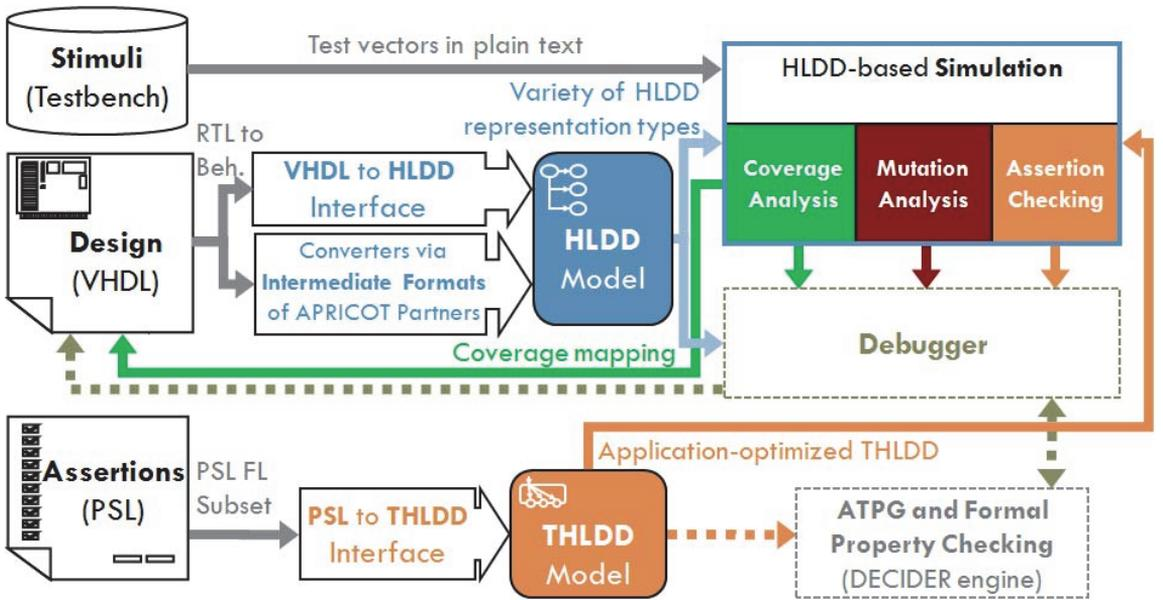
Figure 1. Hardware verification framework APRICOT
