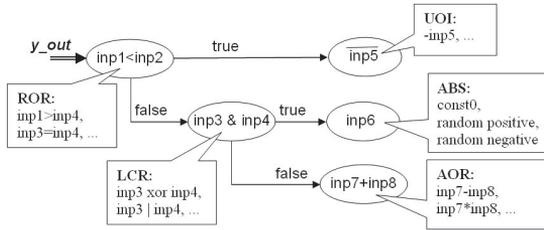
Figure 5. “Key” mutation operators as HLDD perturbations
