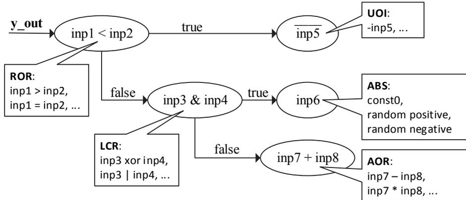
**Figure 3.1. “Key” mutation operators as HLDD perturbations**
