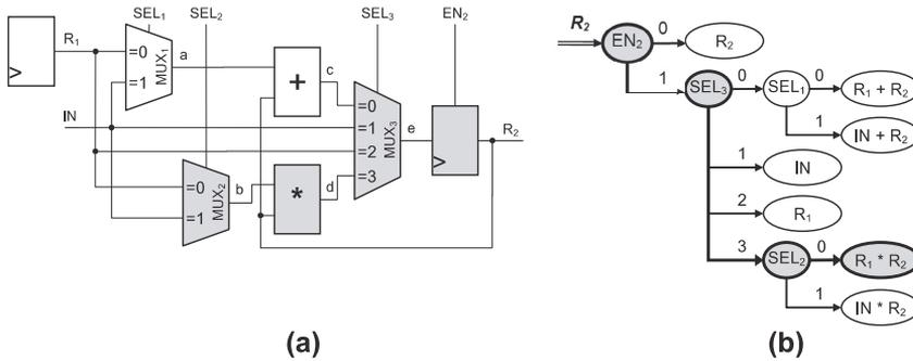
Fig. 3. A datapath of a DUV (a) schematic and (b) HLDD-based representations.
