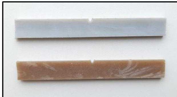
**Figure 2.** V-notched composite samples for Charpy impact test
