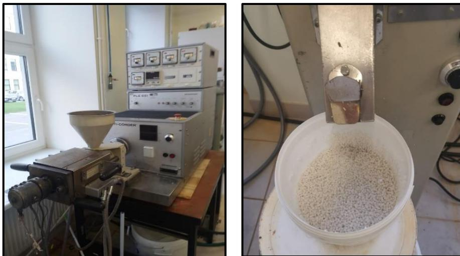
**Figure 5.** Brabender Plasti Corder – PLE 651 twin screw compounder and produced composite pellets
