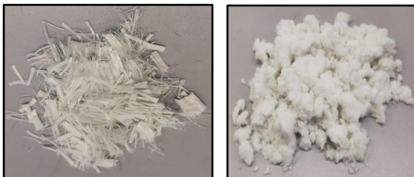
**Figure 3.** Un-milled (left) and milled (right) polyester fibers
