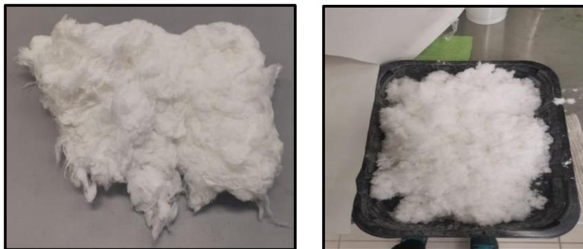
**Figure 2.** Un-milled (left) and milled (right) cotton fibers
