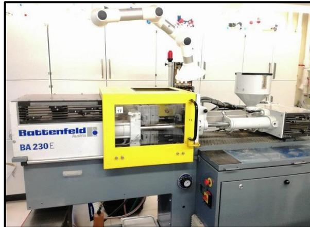
**Figure 6.** Battenfeld Injection molding machinery in TalTech processing lab
