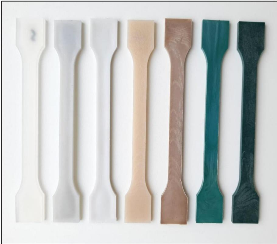
LDPE, PP and RePE composite samples with different fibers and fiber contents
