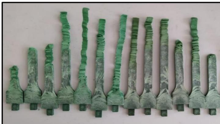
**Figure 7.** Short molding issue during the injection molding of RePE with cotton fiber content of 30%
