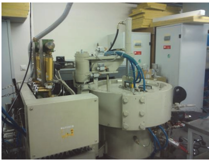
Figure 2.2 SinterHIP machine with an accompanying sintering regime diagram.
