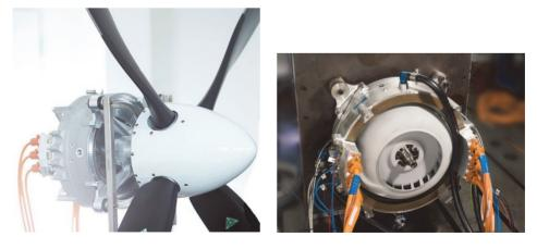
Fig. 1.6. LUFO IV light aircraft motor constructed by Siemens [20].
