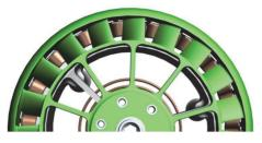
Fig. 2. The air cooling system with an impeller on the rotor.
