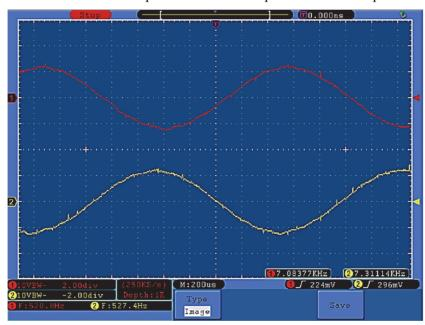
Fig. 5.8. Waveform of the FESM phase voltage  $U_{ph}$  at n = 1500 rpm.
