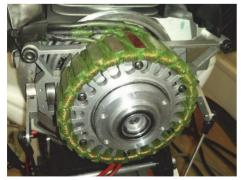
Fig. 3. View of the wound stator.
