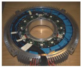
Fig. 1.5. Integrated modular converter with a high power density by PEMC [18].
