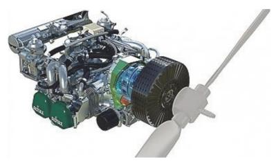
Fig. 1.8. A hybrid-electric drive prototype by Rotax Aircraft Engines [22].
