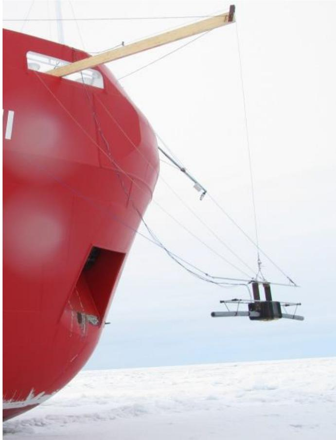
**Figure 5.4 Installation of the EM system (Kujala, 2013)**
