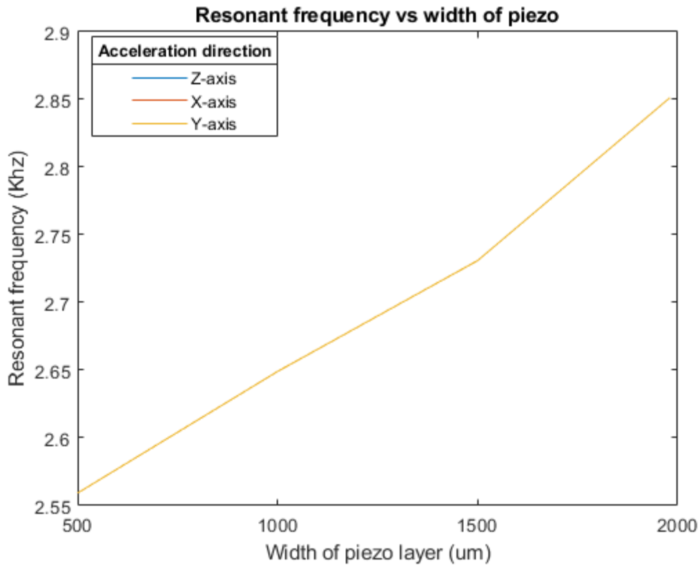
Figure 4. 45. Resonant frequency plot at all three axes acceleration of 1-g with changing width of the piezo layer Voltage sensitivity
