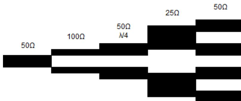
Figure 13. Feed network structure.
