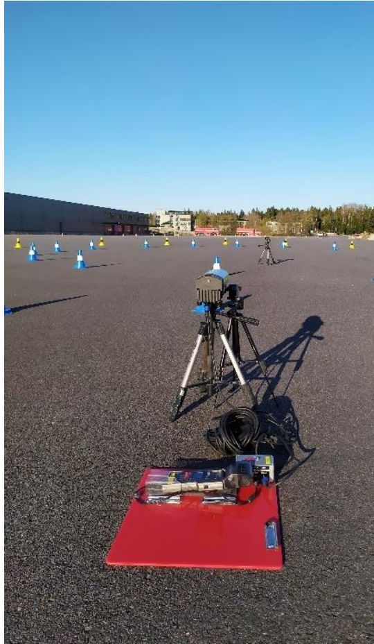
Figure 39. Placement of device under test and verification device on skid pad start/stop line.
