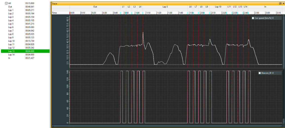
Figure 40. GEMS Data Analysis Pro screenshot of log file including detected lap times.
