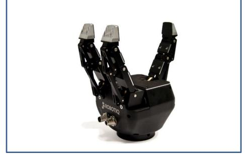
Figure 26 IR End effector/Gripper [18]
