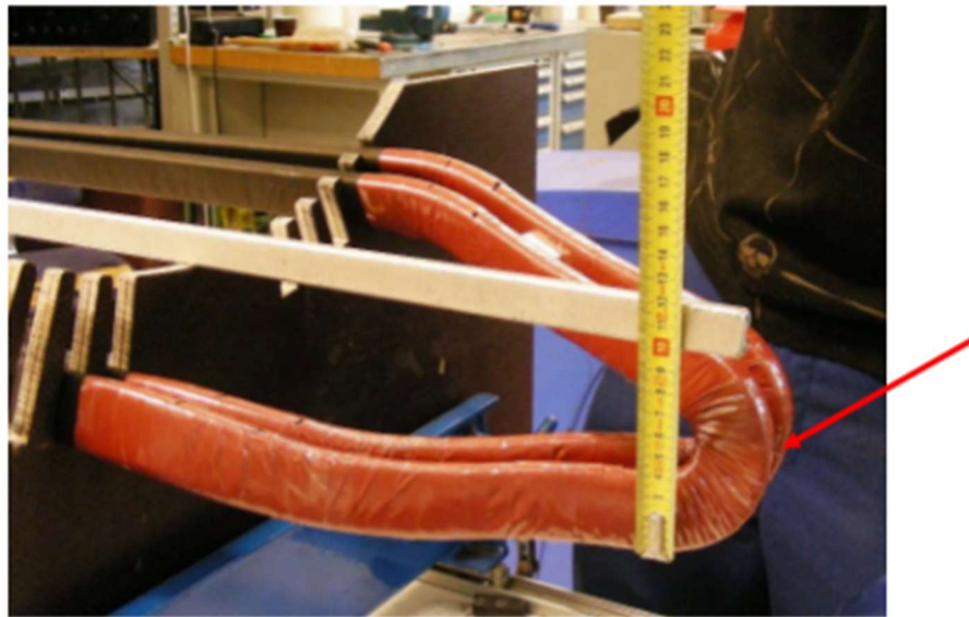
Figure 1.6 Preferred location of chip to identify the production process(marked in red arrow) [5]
