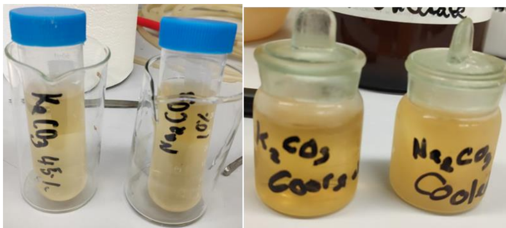
Figure 4.5.2. Induced phase salting out solutions. Left shows the solution after centrifugation and allowing 24 hours for separation. Right shows the same solutions after 24 hours in freezer.
