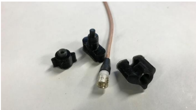
Figure 11. Picture of assembled coaxial cable with 3D printed assembly tools.
