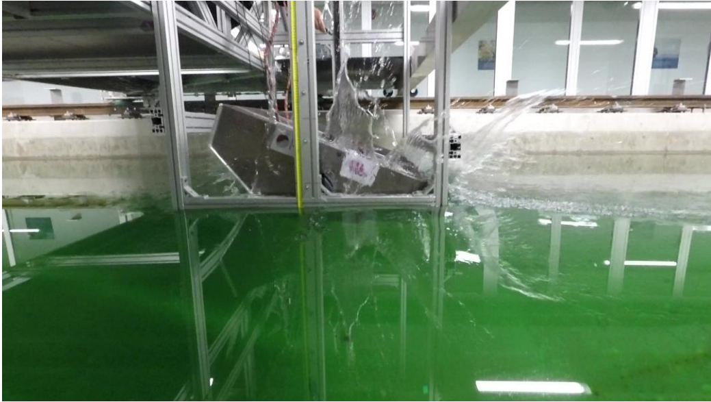
Figure 23. Asymmetrical water entry of the wedge at 50 cm drop height and 25 degree heel angle.
