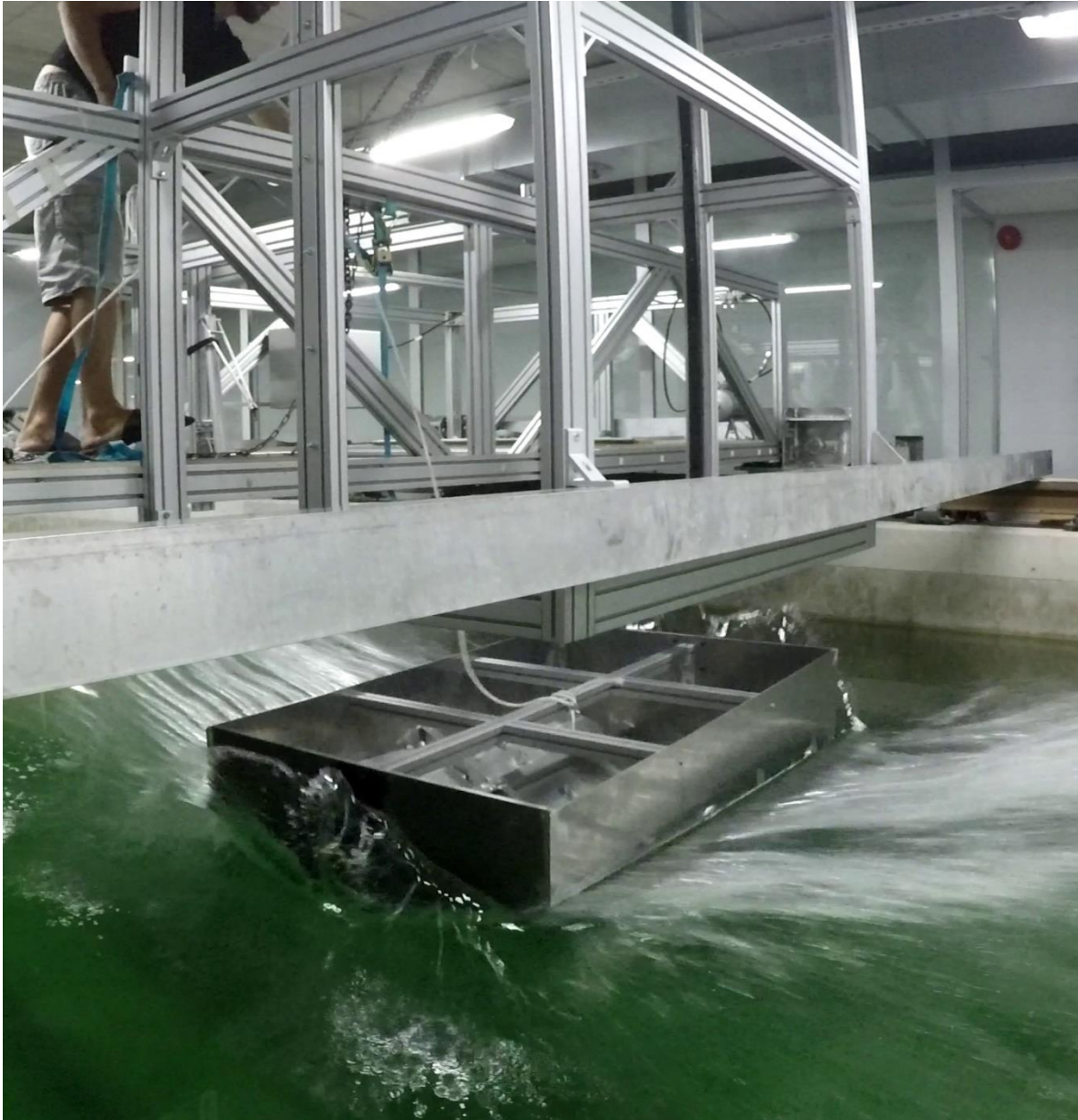
Figure 16. Picture from the initial testing of the setup, without measurement equipment installed.
