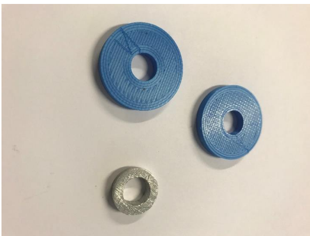
Figure 12. Handmade and 3D printed spacers for mounting pressure sensors.
