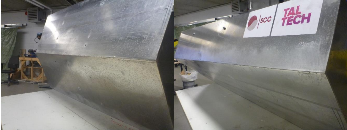
Figure 3. View of the keel and chine of the wedge after sanding and removing the weld beads.
