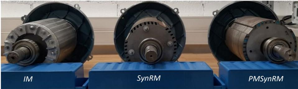
Figure 3-1: Rotors of the tested electrical motor; from the left: industrial IM, the designed SynRM and PMSynRM, respectively.
