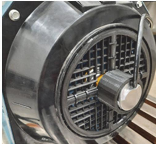
**Figure 4.** The 3D printed holder and coupling for mounting the encoder on the motor.
