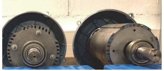
Fig. 4. The rotor structure of the designed SynRM (left side) and the PMSynRM (right side).
