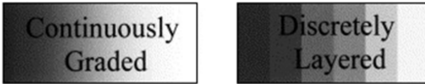
Figure 2.3 Types of graded structures: a) continuously graded structure, b) step-wise graded structure
