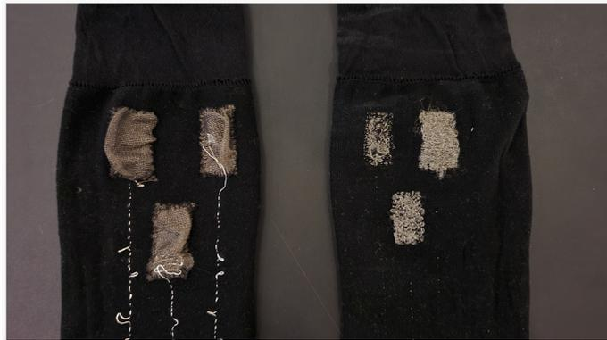
Figure 10. *left: Conductive fabric electrodes with wire covered insulating coat, right: Silver thread electrodes.*
