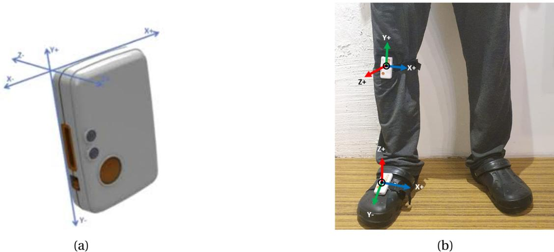
Figure 14. (a) A Shimmer3 device and its reference coordinate system. (b) The alignment between sensor's axes and body reference system.
