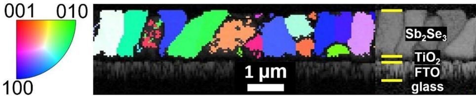
**Figure 25.** EBSD map with orientation distribution of the  $\text{Sb}_2\text{Se}_3$  + SL film (given by false colors, see legend) superimposed on the pattern-quality distribution of the FTO layer. The orientation distribution indicates no pronounced texture of the  $\text{Sb}_2\text{Se}_3$  + SL layer.
