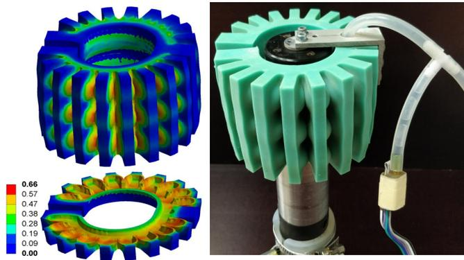
Figure 3.8: The variable stiffness actuator final prototype [Publication III]. The actuator is deformed by increasing its internal pressure by 100 kPa. Left: Equivalent elastic strain levels in FEM simulation. Right: The physical prototype with a fluid intake silicone tube and a pressure measurement module.
