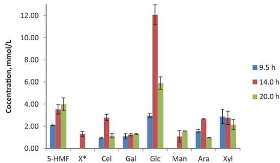
Fig. 2. Detected analytes concentrations in  $C_2$ MIM Cl treated spruce heartwood hydrolysates.
