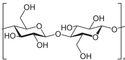
*Figure 1. The cellulose fragment, composed of a linear chain of glucose units linked by  $\beta$ -1,4- glycosidic bonds.*
