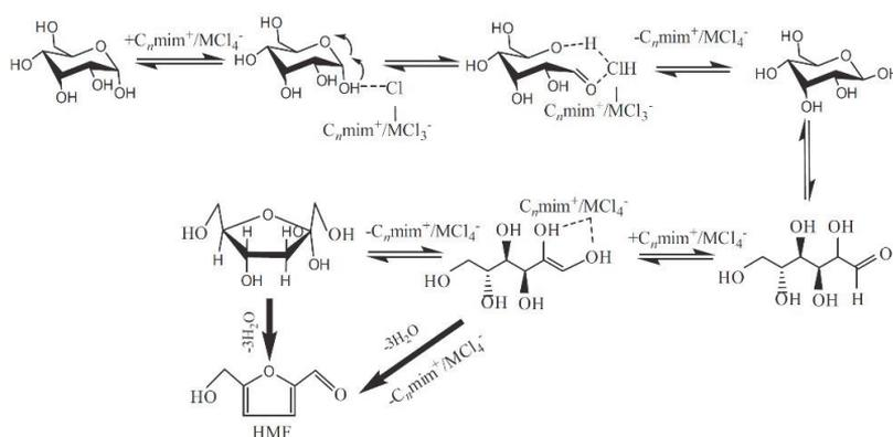
**Figure 2.** Interaction of metal chlorides with glucose to produce HMF in  $\text{C}_n\text{MIM}/\text{MCl}_4$  ( $n = 4$ , 1-*n*-butyl-3-methylimidazolium, [BMIM]Cl; M = Cr, Al and Fe) [35].
