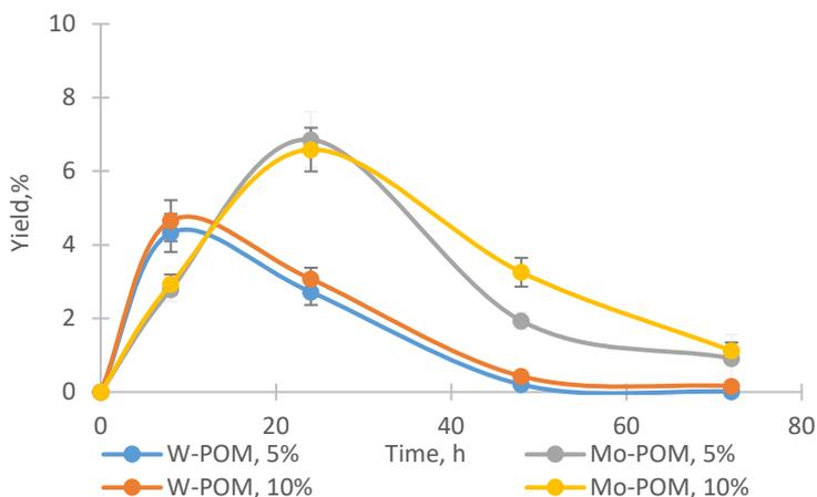
Figure 18. Conversion of cellulose to 5-HMF in [BMIm][Cl] at 120 °C by using tungsten and molybdenum oxide-based POMs at 5 and 10% substrate loading.
