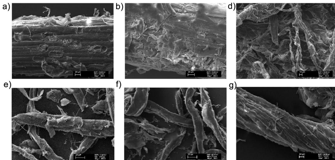
**Fig. 6.** SEM images of  $C_4MIM$  Ac-treated wheat straw samples (at  $100^\circ C$ ) after (a) 1, (b) 6 and (c) 24 h and cellulose samples after (d) 1, (e) 6 and (f) 24 h.
