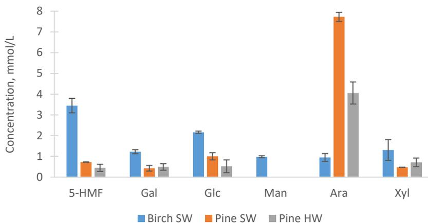
Figure 8. Detected analyte concentrations for [EMIm][Cl] at 100 °C treated birch sapwood (SW, treated for 20h), pine sapwood (treated for 6.5 h) and pine heartwood (HW, treated for 9.5h) samples.
