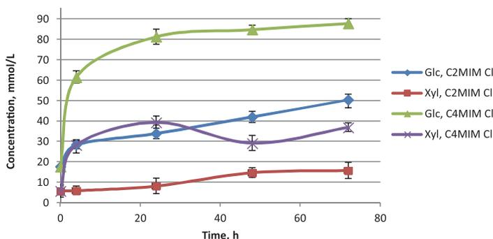
Fig. 5. Dynamics of saccharification process for IL-pretreated wheat straw samples at 110 °C.
