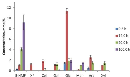
Fig. 1. Detected analytes concentrations in  $C_2$ MIM Cl treated spruce sapwood hydrolysates.
