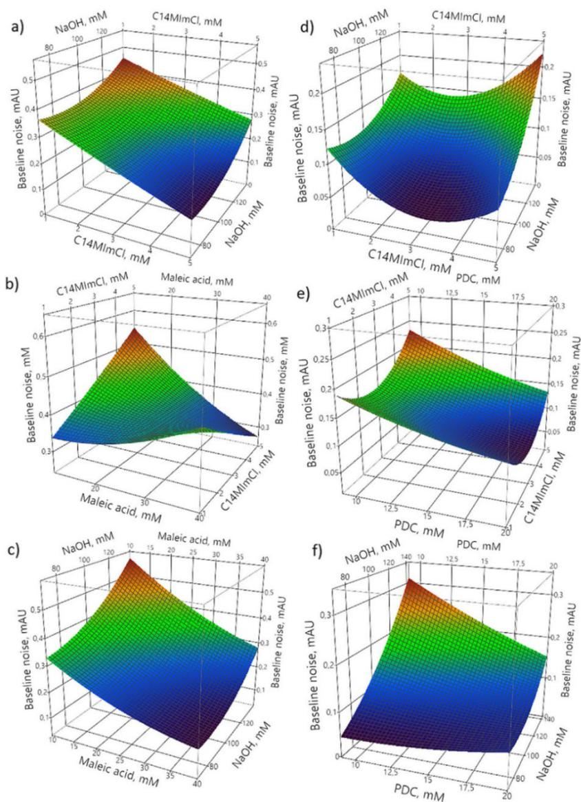
Figure 13. Response surface plots for baseline noise relationships with concentrations of (a) NaOH/[C14MIm][Cl], (b) maleic acid/[C14MIm][Cl], (c) maleic acid/NaOH in maleic acid BGE, (d) NaOH/[C14MIm][Cl], (e) PDC/[C14MIm][Cl] and (f) PDC/NaOH in PDC BGE.
