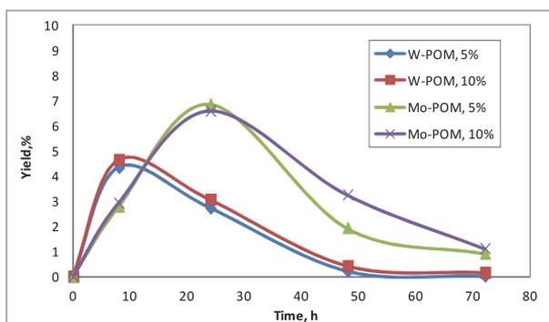
**Figure 4.** Conversion of cellulose to HMF in [BMIM]Cl at 120 °C by using tungsten and molybdenum oxide-based POMs at 5 and 10% substrate loading. Catalyst loading was 10 wt % from cellulose and cellulose loading was 5 or 10 wt % from solvent.
