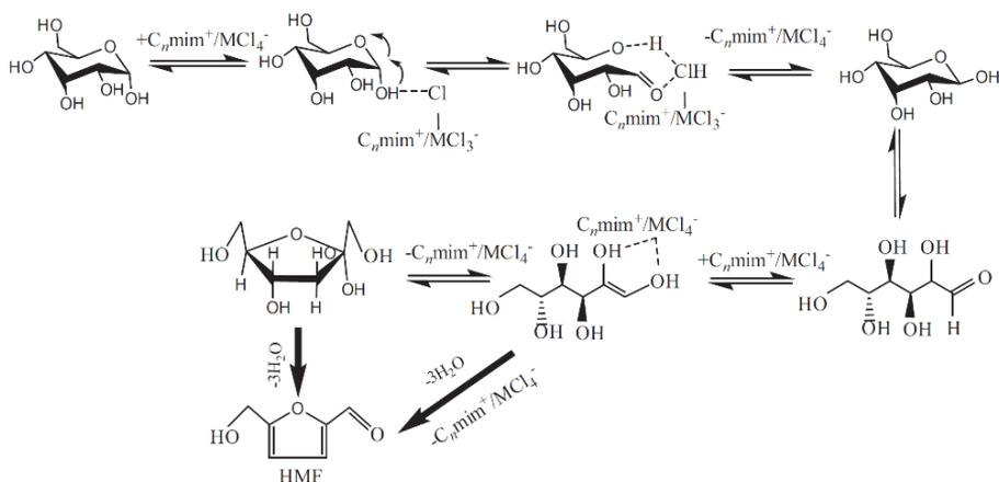
Figure 16. Interaction of metal chlorides with glucose to produce 5-HMF in  $C_n\text{MIM}/\text{MCl}_4$  ( $n = 4, 1$ -*n*-butyl-3-methylimidazolium,  $[\text{BMIm}][\text{Cl}]$ ;  $\text{M} = \text{Cr}, \text{Al}$  and  $\text{Fe}$ ) [30].
