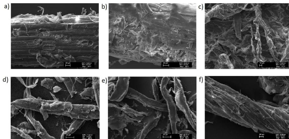
Figure 11. SEM images of [BMIm][OAc]-treated wheat straw samples (at 100 °C) after a) 1, b) 6 and c) 24 h and cellulose samples after d) 1, e) 6 and f) 24h.
