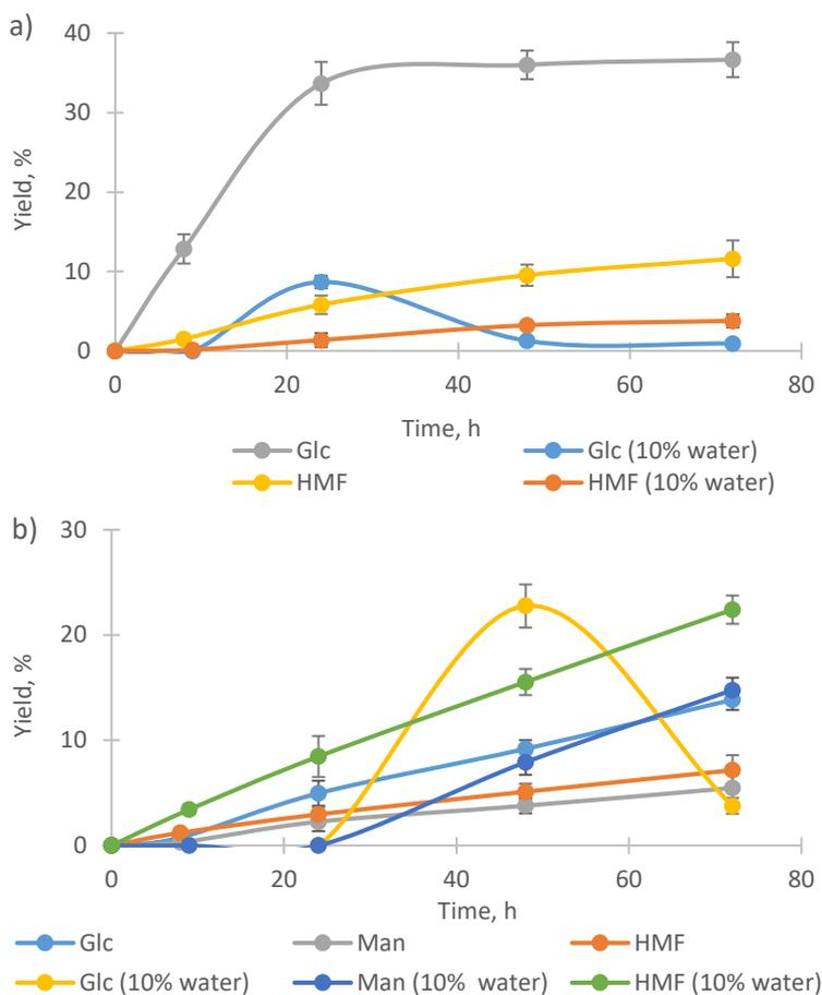
Figure 20. Conversion of cellulose to glucose, mannose and 5-HMF in [BMIm][Cl] at 100 °C in the presence of water (10 wt% of solvent) by using POMs based on (a) tungsten oxide and (b) molybdenum oxide.
