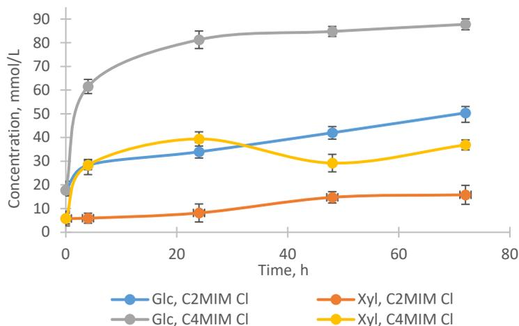
Figure 10. Dynamics of the saccharification process for IL-pretreated wheat straw samples at 110 °C.
