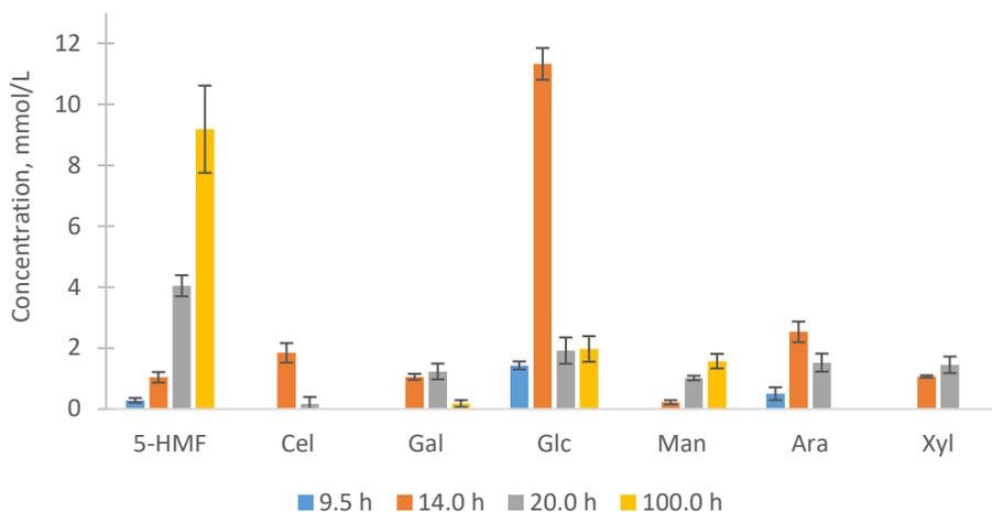
*Figure 6. Detected analyte concentrations in [EMIm][Cl]-treated spruce sapwood samples.*
