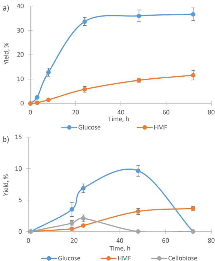
Figure 19. Efficiency of cellulose degradation in [BMIm][Cl] at 100 °C by using phosphotungstic acid hydrate added (a) 20 min before the substrate and (b) 3 h after the substrate.
