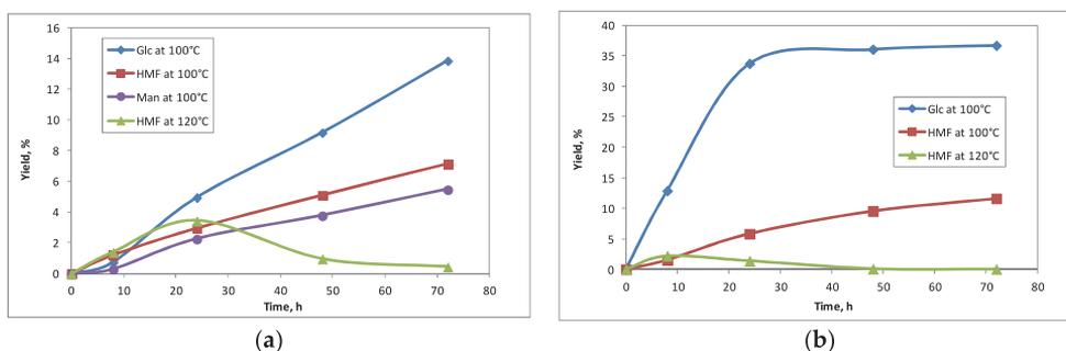
**Figure 3.** Conversion of cellulose to glucose, mannose and HMF in [BMIM]Cl at 100 and 120 °C by using POMs based on (a) molybdenum oxide and (b) tungsten oxide. Catalyst loading was 10 wt % from cellulose and cellulose loading was 10 wt % from solvent.
