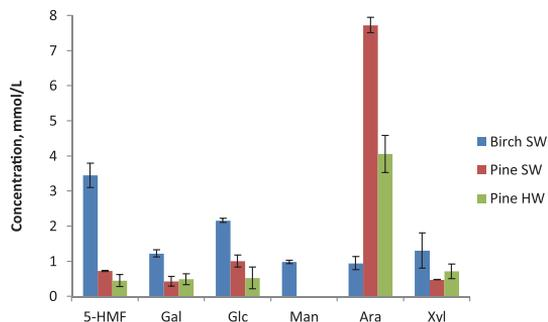
Fig. 3. Detected analytes concentrations for  $C_2$ MIM Cl at  $100^\circ\text{C}$  treated birch sapwood (SW, treated for 20 h), pine sapwood (treated for 6.5 h) and pine heartwood (HW, treated for 9.5 h) hydrolysates.
