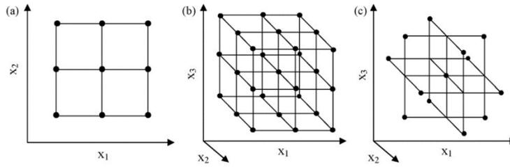
Figure 5. Experimental designs based on the study of all variables on three levels: three-level factorial design for the optimisation of (a) two variables and (b) three variables and (c) BBD for the optimisation of three variables [98].
