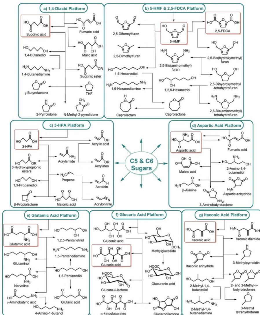
Figure 4. (a) 1,4-diacid, (b) 5-HMF and 2,5-FDCA, (c) 3-HPA, (d) aspartic acid, (e) glutamic acid, (f) glucaric acid and (g) itaconic acid platform chemicals from C5 and C6 sugars [10].
