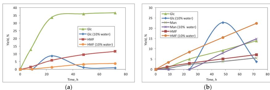
**Figure 6.** Conversion of cellulose to glucose, mannose and HMF in [BMIM]Cl at 100 °C in the presence of water (10 wt % of solvent) by using POMs based on (a) tungsten oxide, (b) molybdenum oxide. Catalyst loading was 10 wt % from cellulose and cellulose loading was 10 wt % from solvent.
