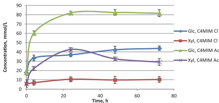
Fig. 4. Dynamics of saccharification process for IL-pretreated wheat straw samples at 100 °C.
