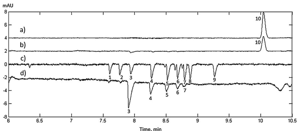
Figure 15. Separation of standards (a, c) and cellulose degradation products (b, d). CE conditions were the following: BGE contained 138.2 mM NaOH, 40 mM maleic acid and 5 mM  $[C_{14}MIm][Cl]$ ; capillary ID 22.5  $\mu$ m; absorbance was measured at 210 (a, b) and 270 (c, d) nm; applied voltage was -21.7 kV. Identification: 1–Xyl, 2–Fru, 3–Glu, 4–Cel, 5–DP3, 6–DP4, 7–DP5, 8–DP6, 9–Suc, 10–5-HMF (analyte concentration: 1 mM of each, except 5-HMF, which was 0.5 mM).
