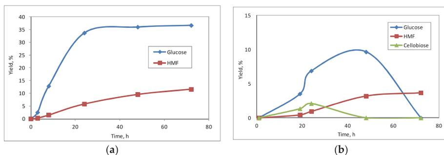
**Figure 5.** Efficiency of cellulose degradation in [BMIM]Cl at 100 °C by using phosphotungstic acid hydrate added (a) 20 min before the substrate, (b) 3 h after the substrate. Catalyst loading was 10 wt % from cellulose and cellulose loading was 10 wt % from solvent.
