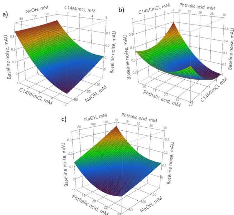
Figure 14. Response surface plots for baseline noise relationships with concentrations of (a) NaOH/[C14MIm][Cl], (b) phthalic acid/[C14MIm][Cl] (c) phthalic acid/NaOH in phthalic acid BGE.
