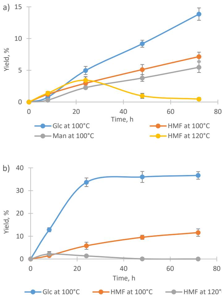
Figure 17. Conversion of cellulose to glucose, mannose and 5-HMF in [BMIm][Cl] at 100 °C and 120 °C by using POMs based on a) molybdenum oxide and b) tungsten oxide.
