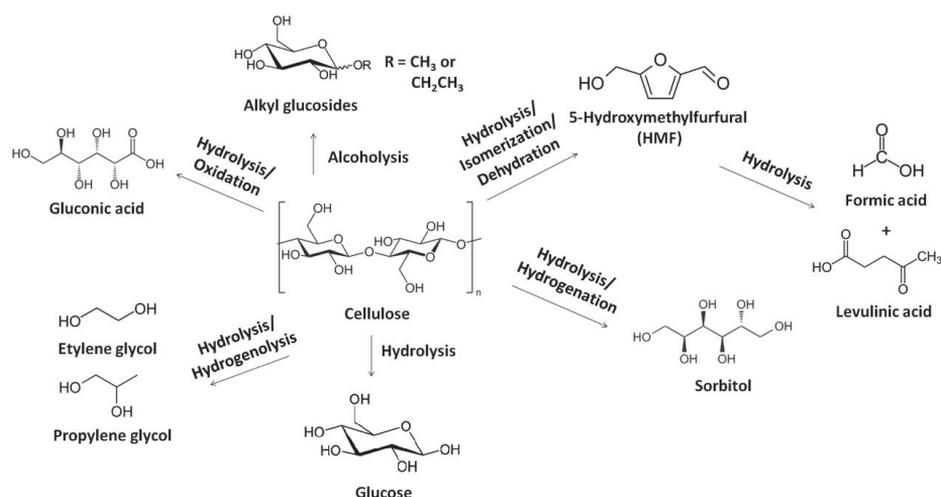
**Figure 1.** Typical platform chemicals produced from the catalytic transformations of cellulose.
