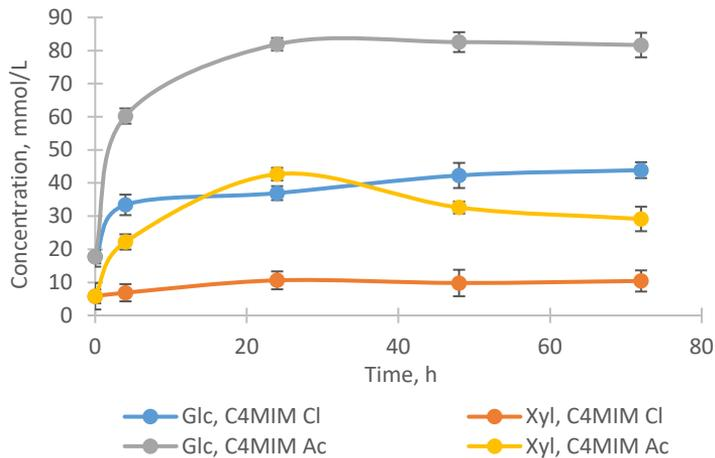
Figure 9. Dynamics of the saccharification process for IL-pretreated wheat straw samples at 100 °C.
