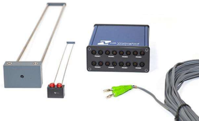
Figure 11: HR Wallingford wave gauge system, wave gauge on the left, amplifier in the centre[17].
