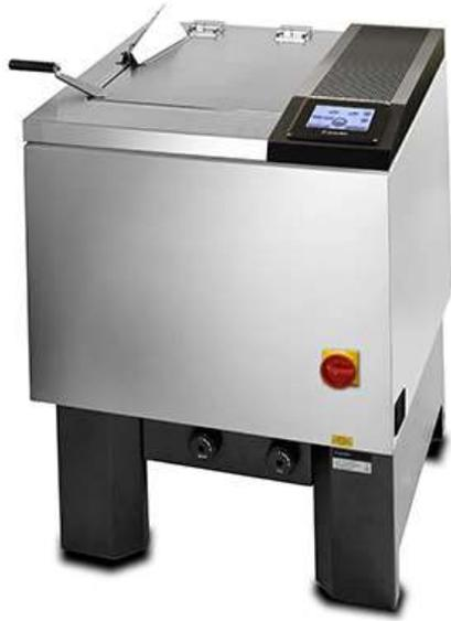
Figure 4.4.1 Testing apparatus for color fastness to laundry testing [58]
