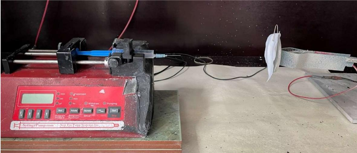
Figure 5.3.1 Electro spraying experiment set up
