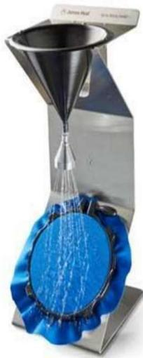
Figure 4.3.1 Spray rate testing machinery setup [56]
