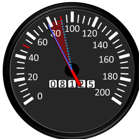
Figure 15. Driver performance–based measure, speed limit keeping ability: light blue dotted line –  $\Delta v_p$ ; blue solid line –  $\Delta v$ ; red surface –  $\Delta v_r$ .
