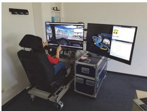
Fig. 2. Driver-in-the-loop experiment simulator.
