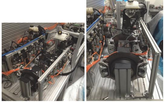
Fig. 3. Different views of the EHB hardware-in-the-loop testbed.
