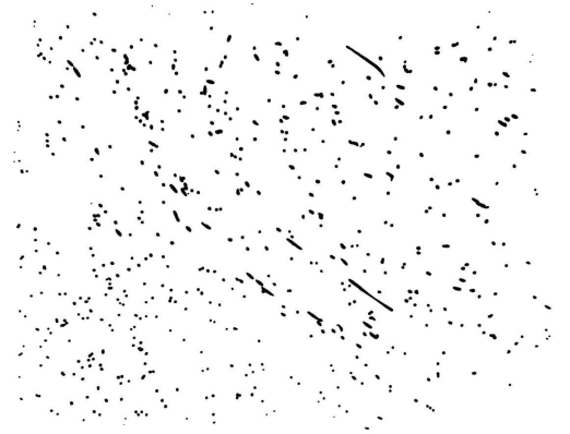
Fig. 2. Image of a slice. (a) Filtered image of a slice; bright spots are fibres. (b) Processed image of a slice in binary format; black spots are fibres.
