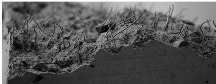
Fig. 1. Steel fibre reinforced concrete after a fracture test.
