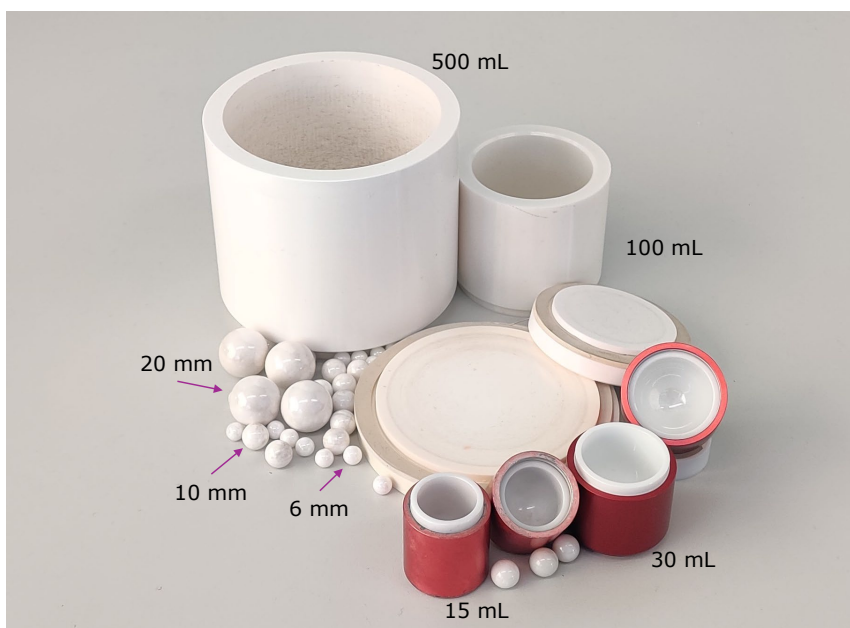
Figure 12. Various \text{ZrO}_2 jars for shaker and planetary mills available in our laboratory and used in the current work.
