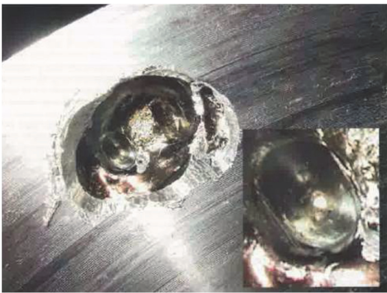
Fig. 1.6. Broken rotor bar due to defective casting [5].
