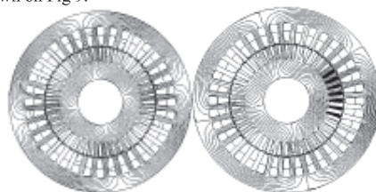
Fig. 9 Magnetic field distribution in the cross section of a 3 kW induction motor at nominal load operating condition: left – healthy rotor cage, right – faulty rotor cage with seven broken bars (shaded) [15]
