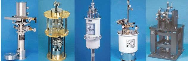
10 mK to 800 K      LHe/LN<sub>2</sub> Cryostats
