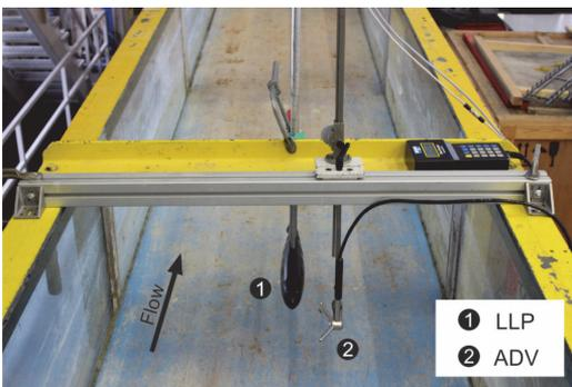
FIG. 3. Setup in the open channel flume (experiment 2), flow direction is given by the arrow. The view is from above facing downstream where the LLP is placed in the center of the flume and adjusted only in the vertical direction. The ADV is positioned such that the sampling volume is located 10 cm in front of the LLP nose sensor,  $P_0$  (Figure 1).
