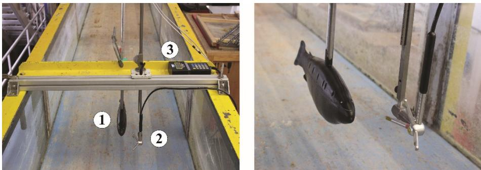
*Figure 2.2 Left: typical experimental setup at the open top flow tunnel in the University of Stuttgart. 1 – Lateral line probe, 2 and 3 – acoustic Doppler velocimeters probe and data logger. Right: close up photo of the probes.*
