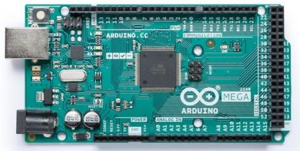
Figure 4.6 Arduino Mega 2560 [30]
