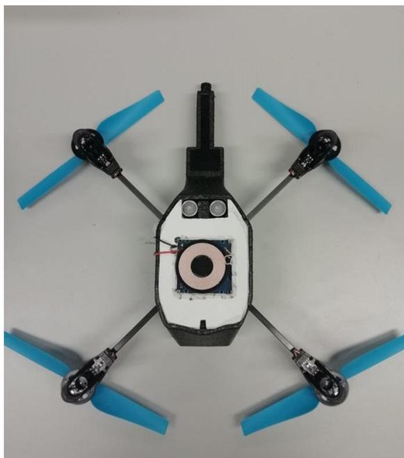
Figure 3.11 Wireless power receiver placed under the drone
