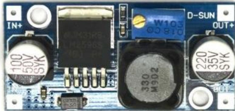
Figure 3.8 LM2596 DC-DC Step-down buck converter [27]
