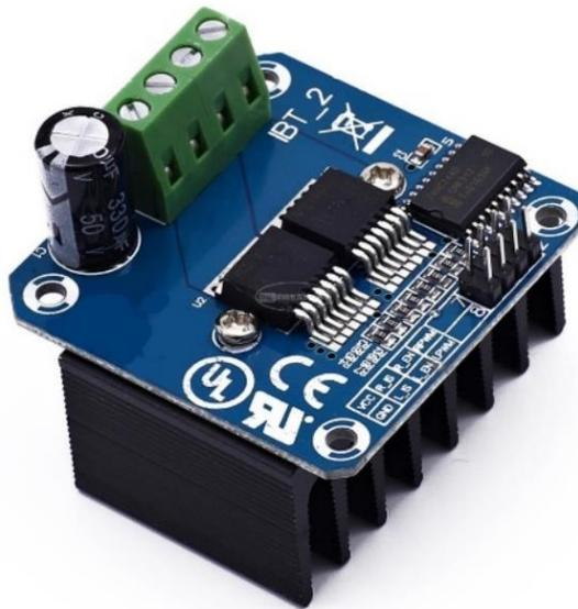
Figure 4.7 BTS7960 - 43A Motor drive
