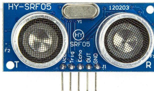
Figure 4.11 SRF05 Ultrasonic distance sensor [37]
