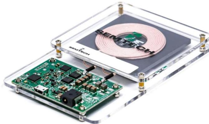
Figure 3.4 Semtech TSDMTX-24V3-EVM transmitter [22]
