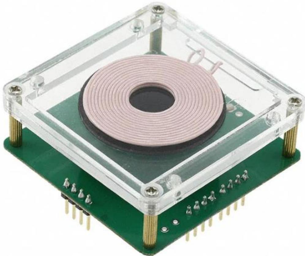
Figure 3.6 TSDMRX-19V/40W-EVM receiver [23]
