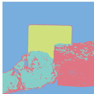
Fig. 12. HSI image classification result showing Tourmaline in cyan and Apatite in red.
