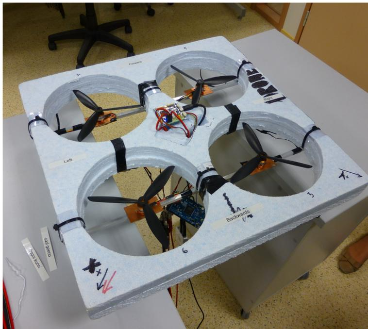
Figure 6. *Frame Design. First Design of Polystyrene Foam.*
