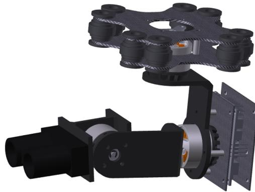
Figure 36. *LIDAR-based Environmental Perception System's Model.*
