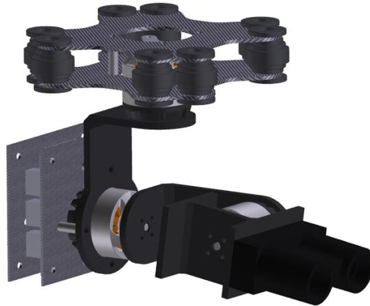
Figure 33. *Design for Stabilizing System.*
