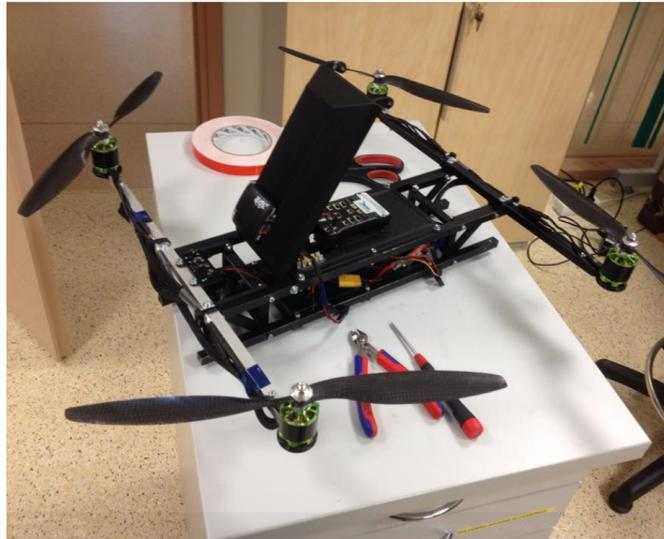
Figure 11. *Frame Design. Final Frame.*
