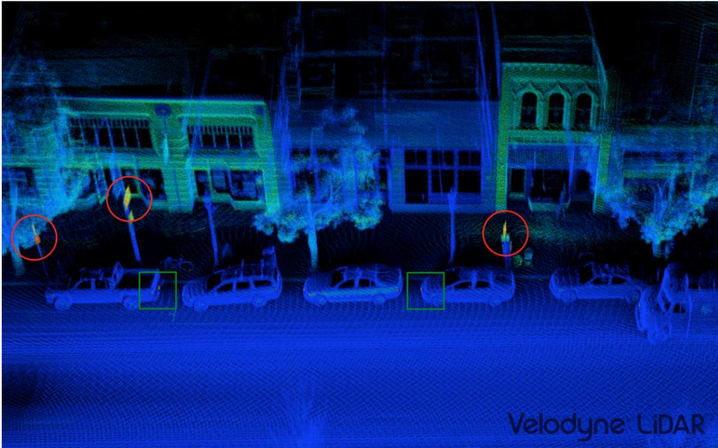
Figure 27. *Environmental Perception. Velodyne HDL-64E LIDAR Scan Example [2].*
