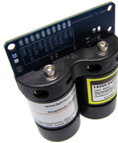
Figure 31. *OSLRF-01 LIDAR Sensor.*
