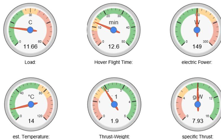
Figure 12. *Estimated results for final model with Turnigy 800 KV 12"x4.5".*
