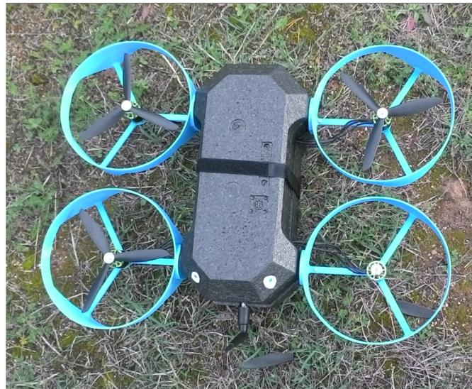
Figure 8. *Frame Design. Second Design – 3D Printed Frame with Polystyrene Foam.*
