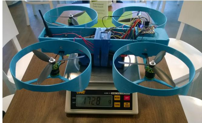
Figure 7. *Frame Design. Second Design – 3D Printed Frame.*
