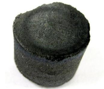
**Fig. 3.1** Typical Ø18 mm PLD target, sintered from CZTS monograin powder.
