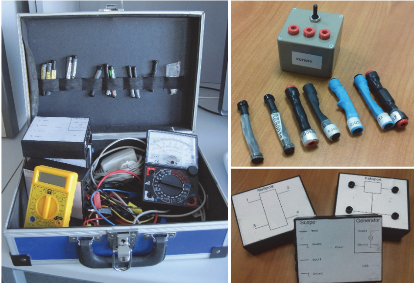
Figure 3.1: HomeLabKit for bachelor students and some of its components
