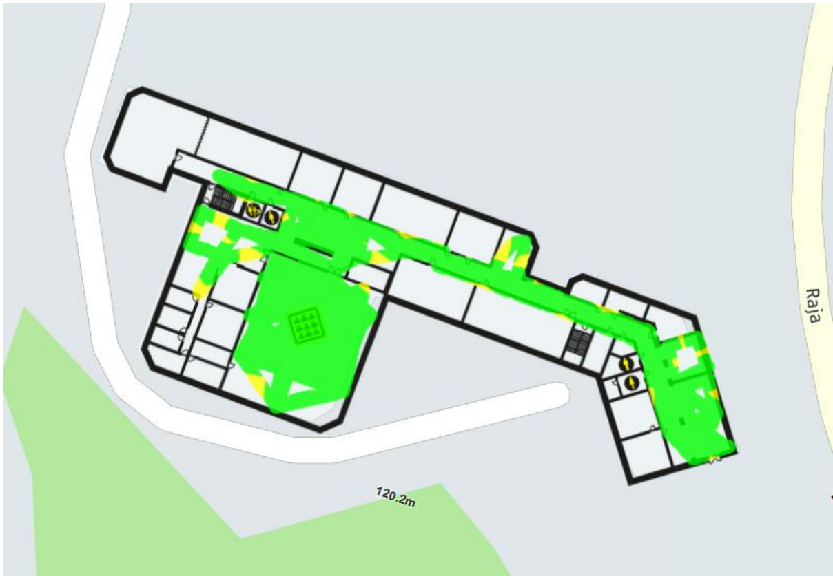
Figure 7 Recorded magnetic field after mapping
