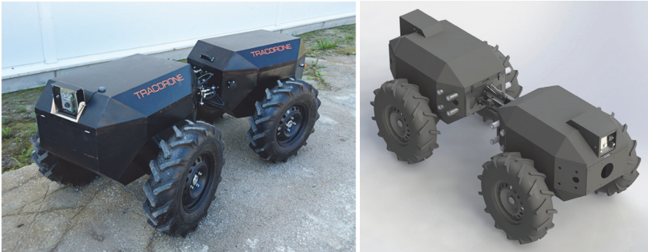
Figure 5.3 Articulated steering hydraulic drive electric UGV Tracdrone and its computer aided design (CAD) model.
