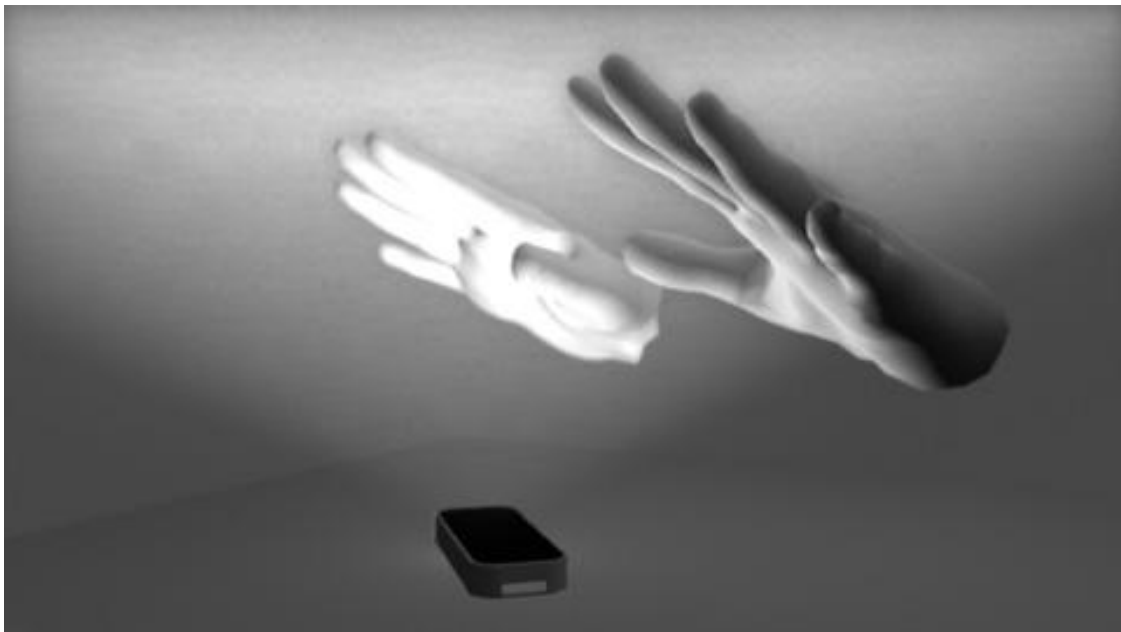
Figure 2. The Leap Motion controller's view of your hands [2]
