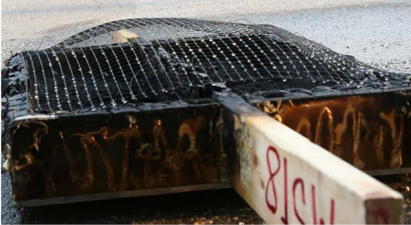
*Figure 3-16. Bending of the steel net occurred in the specimen that was prepared for Test 17.*
