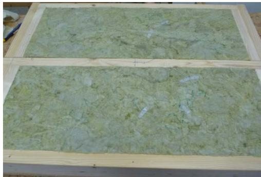
Figure 3-6. A mineral wool product positioned in a wooden frame.
