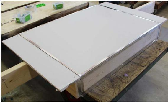
Figure 3-7. Gypsum plasterboard as fire protection mounted on a specimen.
