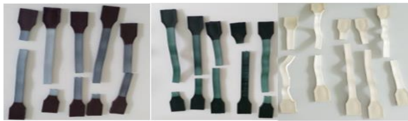
Figure 3.5 Tensile tested samples at 400 h (Author's photo)
