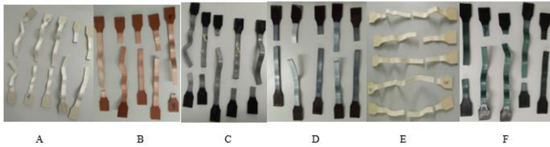
Figure 3.4 Tensile tested samples at 300 h (Author's photo)
