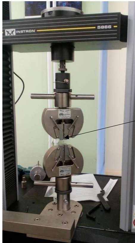
Figure 2.5 Tensile testing machine (INSTRON 5866) (Author's photo)
