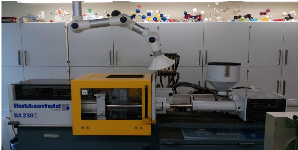
Figure 2.2 Injection moulding machine (Author's photo)
