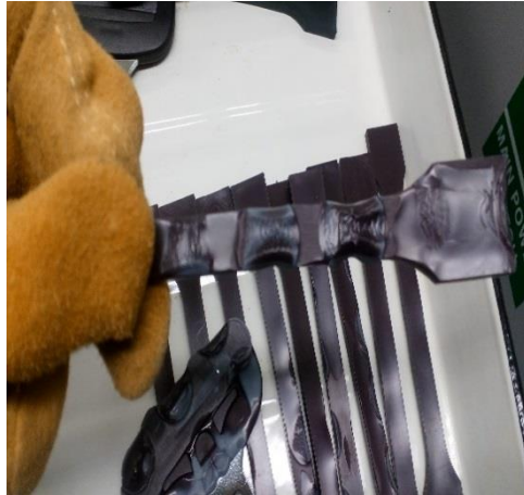
Figure 2.4 Damson coloured sample partially melted after 100 h (Author's photo)
