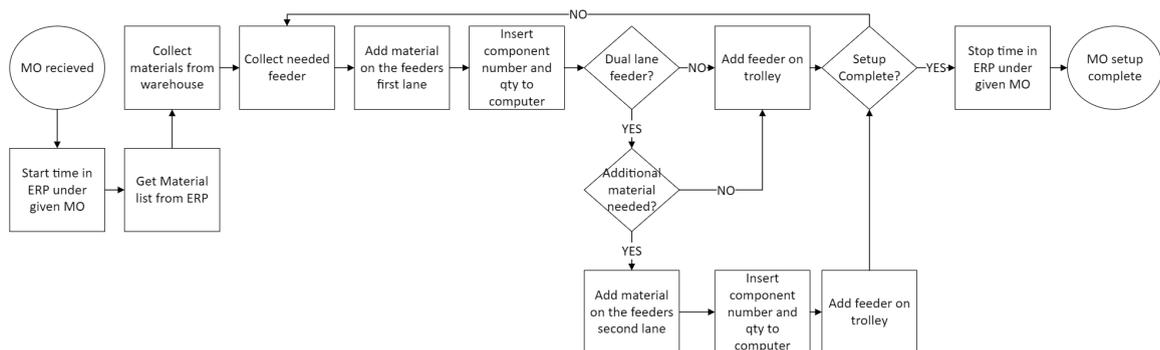
Figure 3.4 Kitting and preparation process
