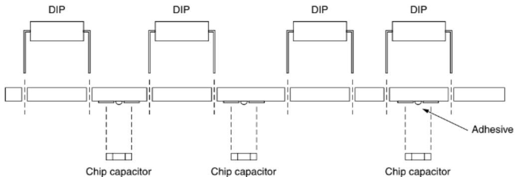
Figure 2.2 Schematic of type III surface mount boards [3]
