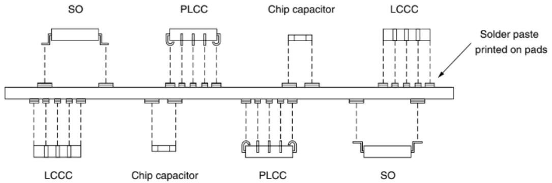
Figure 2.1 Schematic of type I surface mount boards [3]
