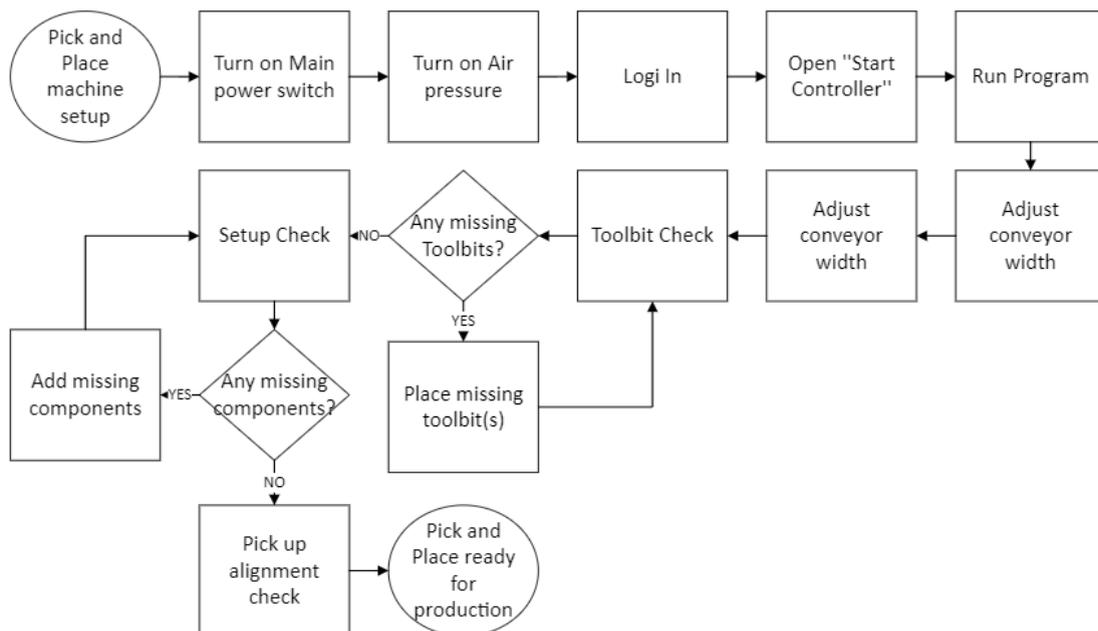
Figure 3.3 PnP Setup Process
