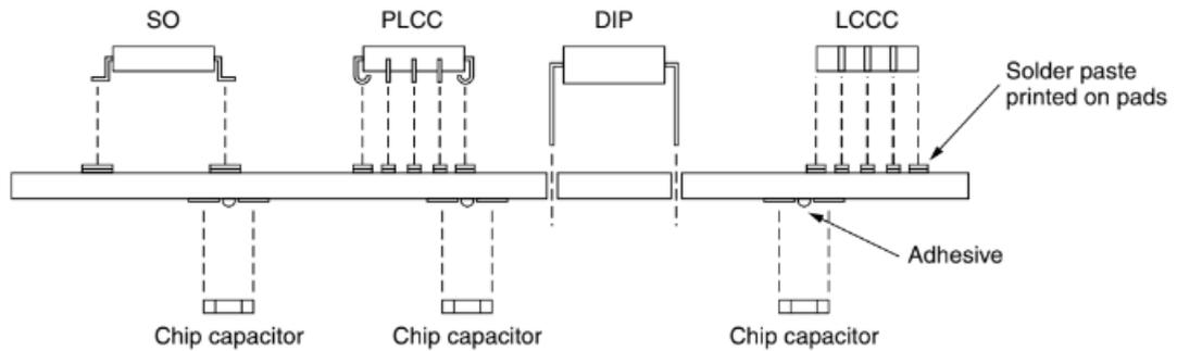
Figure 1.12 Schematic of type II surface mount boards
