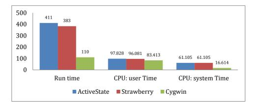
Figure 4. Perl performance using looping rule, With Disk I/O
