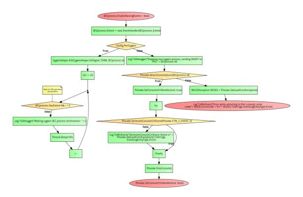
Figure 10. SECwin flowchart: Terminating SEC gracefully
