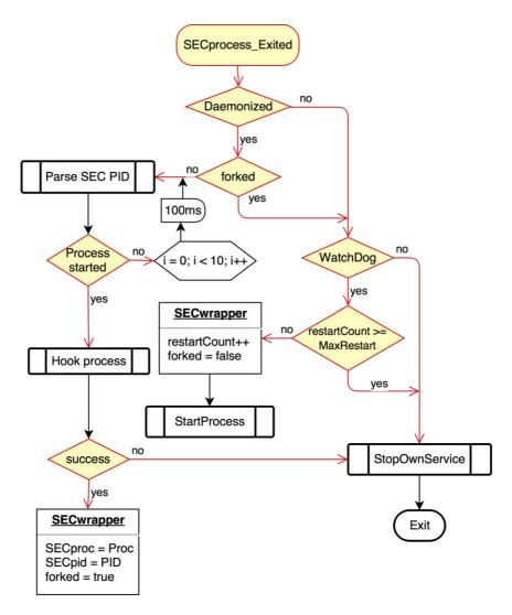
Figure 11. SECwin flowchart: Handling unexpected termination
