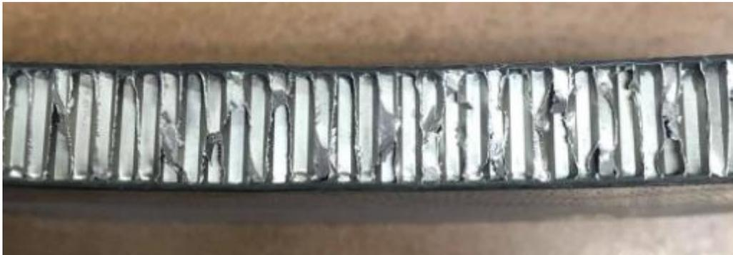
Figure 4.3 Cross-section of car body. Credit: Kaarel Haavajõe
