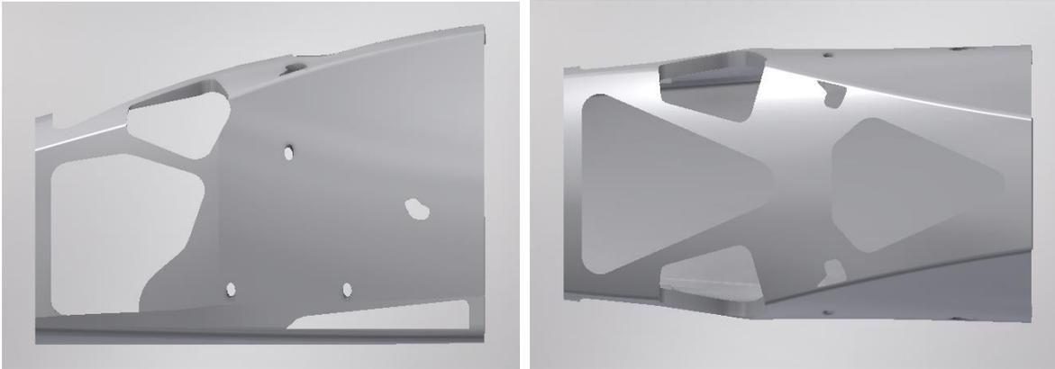
Figure 5.8 New model base generated through topology optimization
