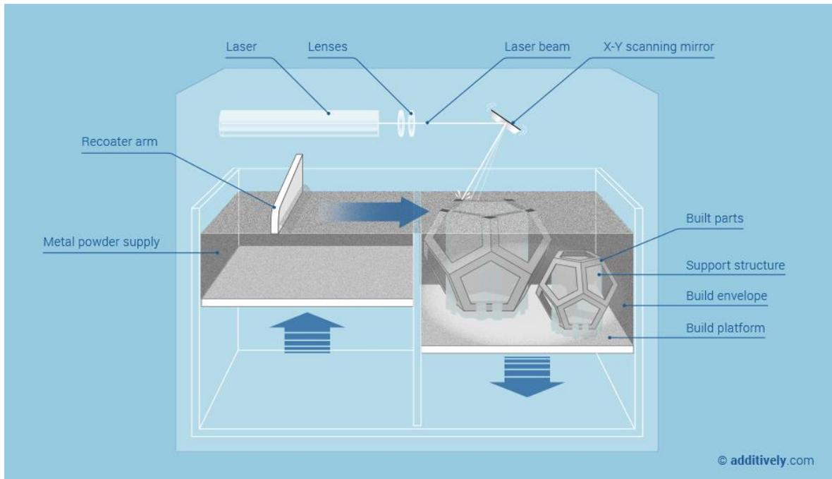
Figure 3.3 SLM principle [13]
