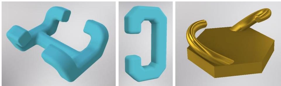
Figure 5.28 Concept 2 open links in blue and concept 3 open link in gold
