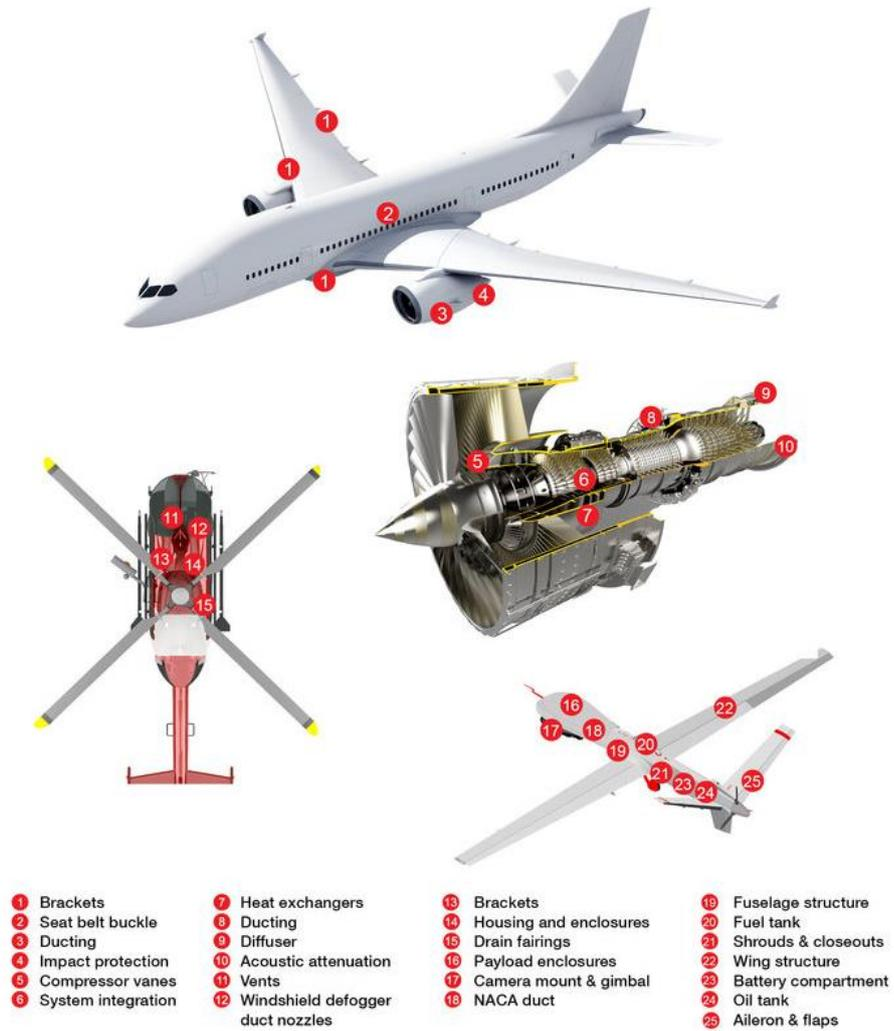
Figure 3.14 Aerospace AM applications [30]
