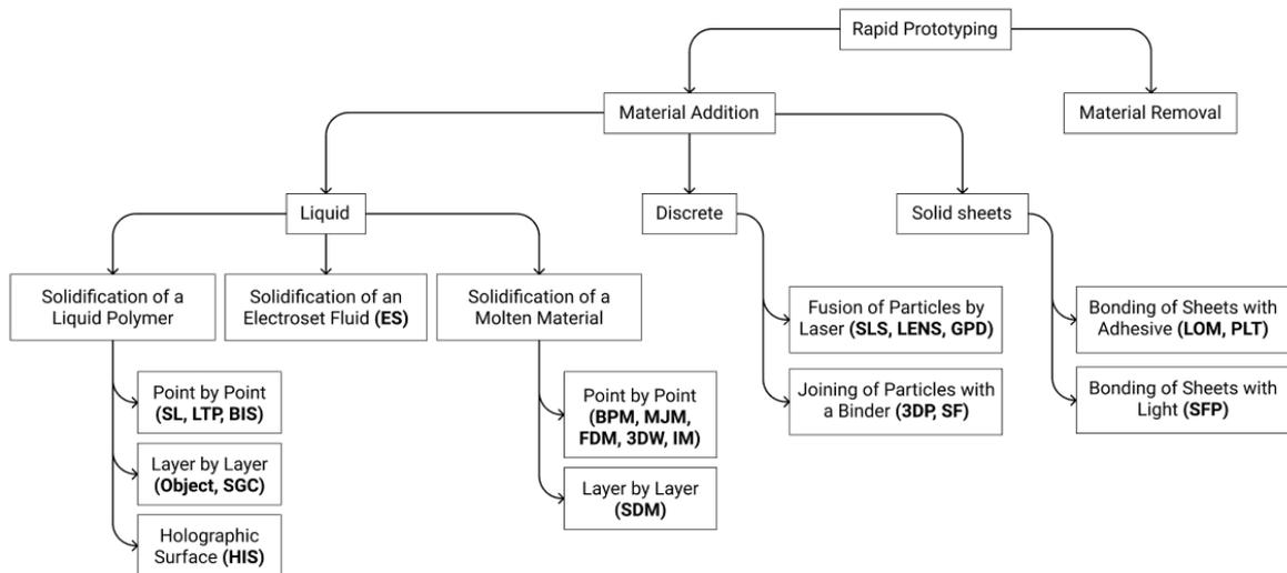
Figure 3.2 AM classification based on raw material state. (Source: [6]. Reproduced from *Additive manufacturing: fundamentals and advancements*)
