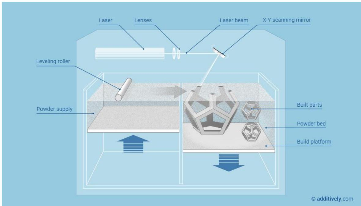
Figure 3.4 SLS printer [16]
