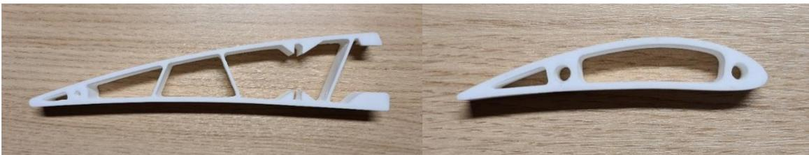
Figure 4.10 An open and closed structure for wings. Author's photos
