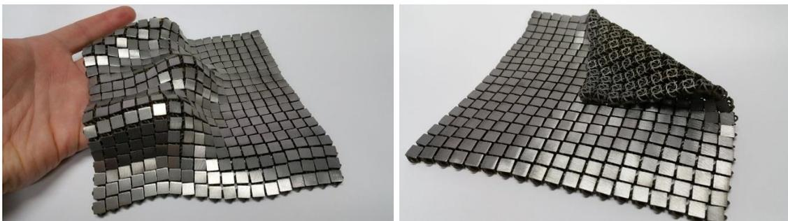
Figure 3.23 NASA 3D printed metal fabric [43]
