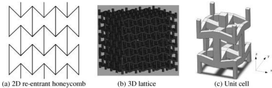
Figure 3.6 Re-entrant honeycomb auxetic structure [19]
